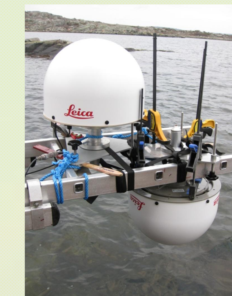
Figure 5: Experimental setup for the GNSS-based tide gauge.
