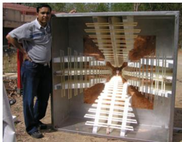
Figure 1: Manufactured Eleven Feed
