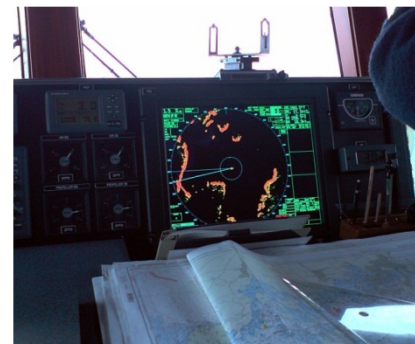
Fig. 1. The alidade of the pelorus in the front window of a Swedish navy ship serves as a reminder of the next course.
