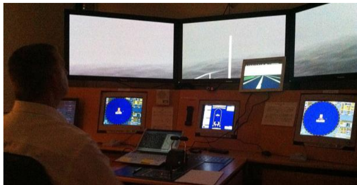
Fig. 3. User testing of a “3D chart” in a smaller simulator. A rescue boat driver is conducting a parallel search in bad visibility. The search pattern he is following is displayed on the 3D chart in the window.
