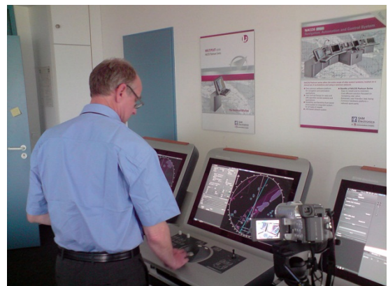
Fig. 6. A pilot is testing the new interface to the SAM NACOS Platinum radar. Video camera records comments as the user "thinks out loud".
