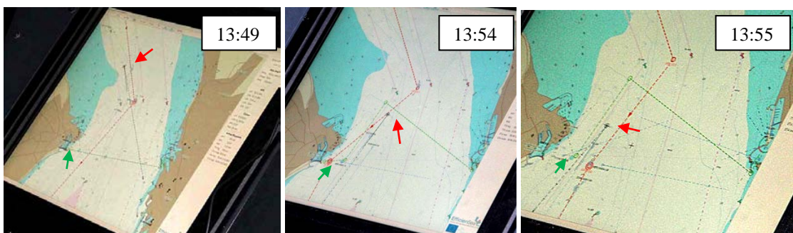
Fig. 5. An example of negotiating a conflicting situation using intended routes: Own ship T.C.Gleisner (red pointer) is the black symbol somewhat west of her (red) track in the upper left part of the screen in the left Figure. Tycko Brahe's (green pointer) green track shows, in the left Figure, that she first intends to go straight across the strait in front of T.C.Gleisner. In the middle T.C.Gleisner has published her intentions to go astern of Tycko Brahe (in accordance with COLREGS) by inserting a new waypoint and moving it west. This will bring T.C. Gleisner's track very close to the port entrance and in the right Figure Tycko Brahe has offered to yield and go astern of T.C.Gleisner, who has accepted by moving her waypoint back to her original track. Photos of T.C.Gleisners ECDIS screen 13:49, 13:54 and 13:55 respectively.
