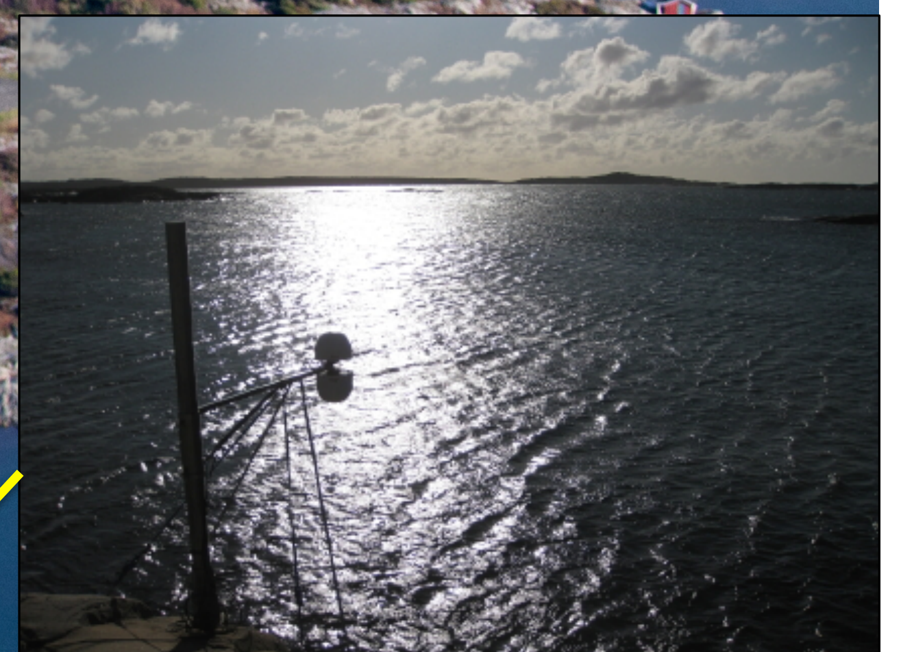
9. The GNSS-based tide gauge operating since 2011.
