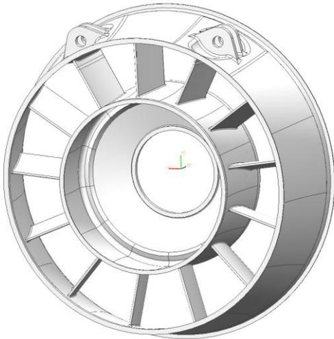
FIGURE 5: Turbine structure CAD model
