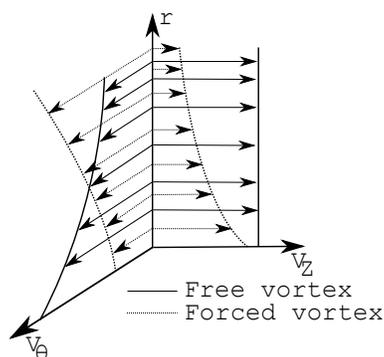
Figure 2: Free and forced vortex velocity distribution [8].
