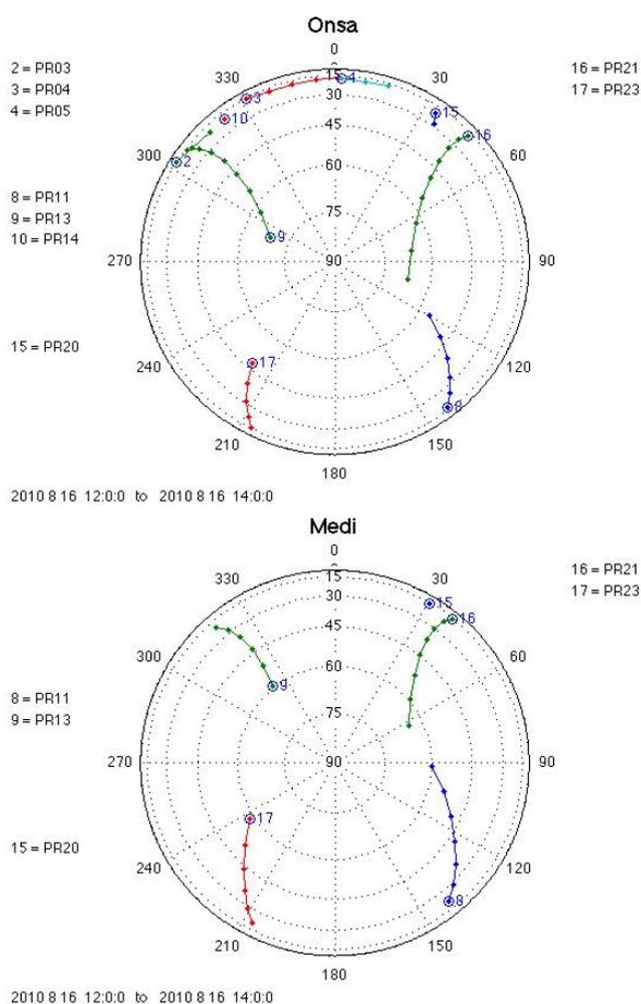
**Figure 1: Sky-plots for Onsala (top) and Medicina (bottom) used for planning the observations on August 16, 2010. The plots are based on predicted orbits provided by the Center for orbit determination in Europe (CODE).**
