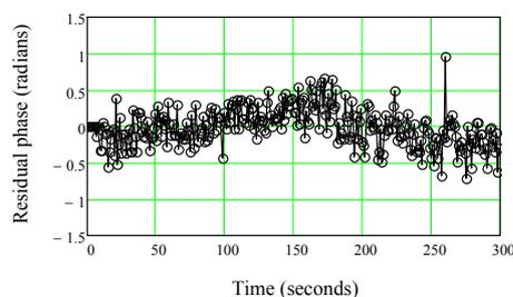
**Figure 3: Residual phase of the fringe. Clock offset calibration accuracy is at a level of 0.2 ns, clock rate offset determination accuracy is better than 0.05 ps/s. Phase noise is at a level of 0.2 radians at 1 s sampling.**
