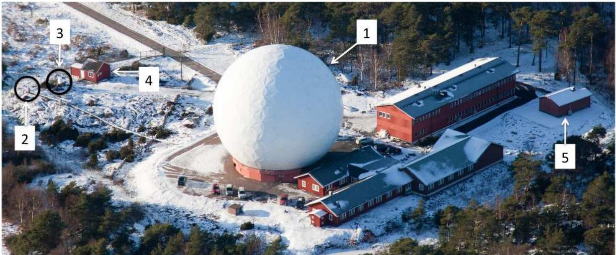
Figure 1. Aerial photo taken in December 2010. Shown are: (1) the radome enclosing the 20-m radio telescope used for geodetic/astrometric VLBI, (2) the IGS antenna, (3) the water vapor radiometer Astrid, (4) the old gravimeter house, (5) the new gravimeter house, and additional office and laboratory buildings.
