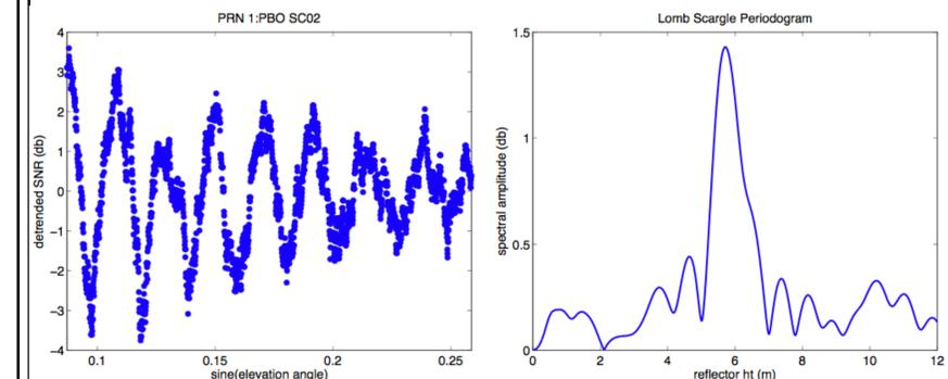
Left: L2C SNR data for PRN 1 between elevation angles of 5 and 15 degrees; right: Lomb Scargle periodogram for these data, showing a strong reflector ~6 meters below the antenna phase center.
