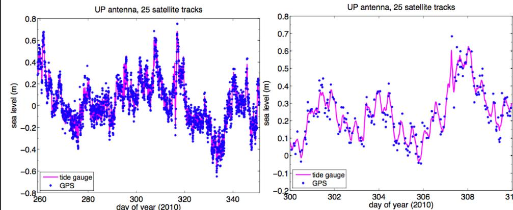
Each blue point represents sea level estimated for a single rising/setting GPS data arc. The magenta line is a linear combination of the Ringhals and Göteborg tidegauge data. RMS agreement between the tidegauge data and the GPS reflections is 4.5 cm.
