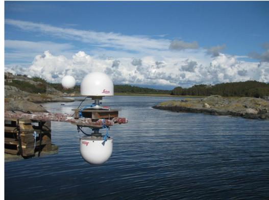
modified to emphasize Left-Handed Circularly Polarized energy from below the horizon. Both the UP and DOWN receivers were tracking at 1-Hz. Rather than a geodetic installation, where the antenna is pounded into bedrock, these antennae have been deliberately set above the local sea surface. There was no *in situ* tide gauge at OSO during the period of this experiment, September-December 2010. However, tide gauges at Ringhals (18 km) and Göteborg (33 km) are available for comparison.
