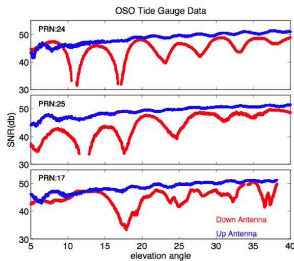
The SNR data for the UP and DOWN antenna are significantly different. The UP antenna primarily shows the effect of the direct signal, with strong signal strength consistent with code-tracking. The DOWN antenna shows deep fades associated with the reflections. The distance between the fades provides the information about the height of local sea level. The DOWN SNR data are consistent with previous studies of Hannah [2001].
