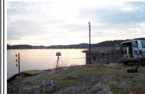
The EarthScope Plate Boundary Observatory (PBO) GPS tide gauge at SC02 (Friday Harbor, WA) is an example of a single antenna-receiver GPS tide gauge. The antenna is a geodetic choke-ring model that is optimized to receive RHCP energy from above the horizon. The receiver is a Trimble NetRS, and the default PBO sample interval is 15 sec. Unlike the OSO GPS tide gauge, the PBO site has been installed in bedrock.
