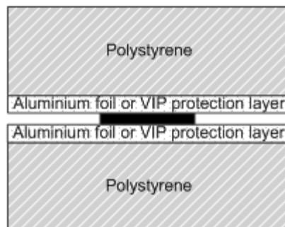
Figure 2. The setups for determination of the protection layer's influence.
