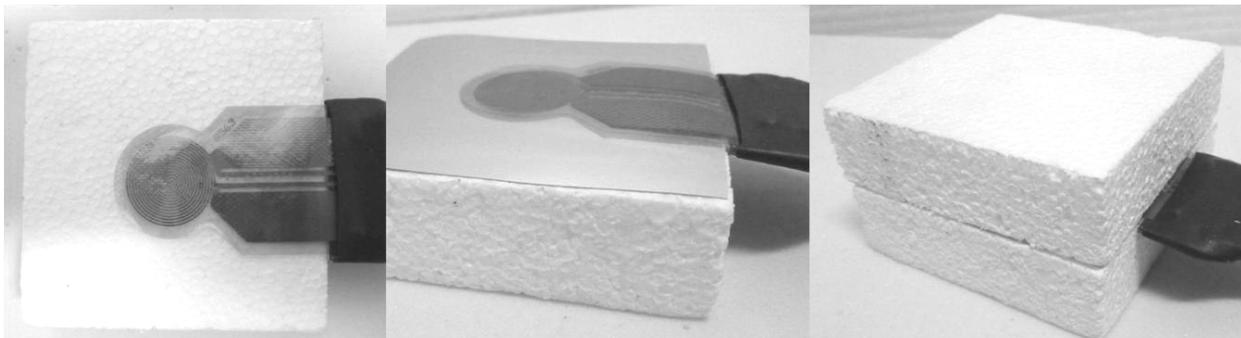
Figure 1. a) TPS sensor on polystyrene, b) TPS sensor on polystyrene covered with aluminium c) TPS sensor clamped between two samples of polystyrene.
