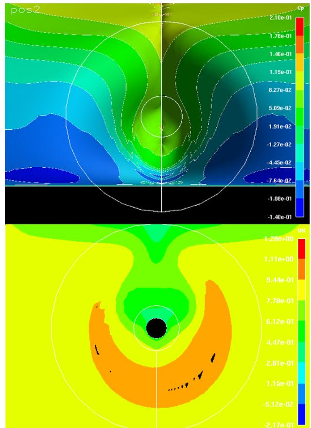
Figure 10: Pressure distribution on hull and axial velocity just upstream the propeller for pos2 with LAP
