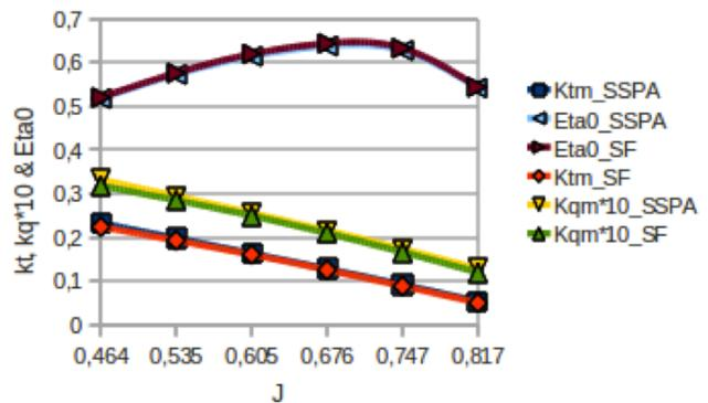
Figure 13: Comparing open water results for the original propeller using LL and experimental data (SF: SHIPFLOW)
