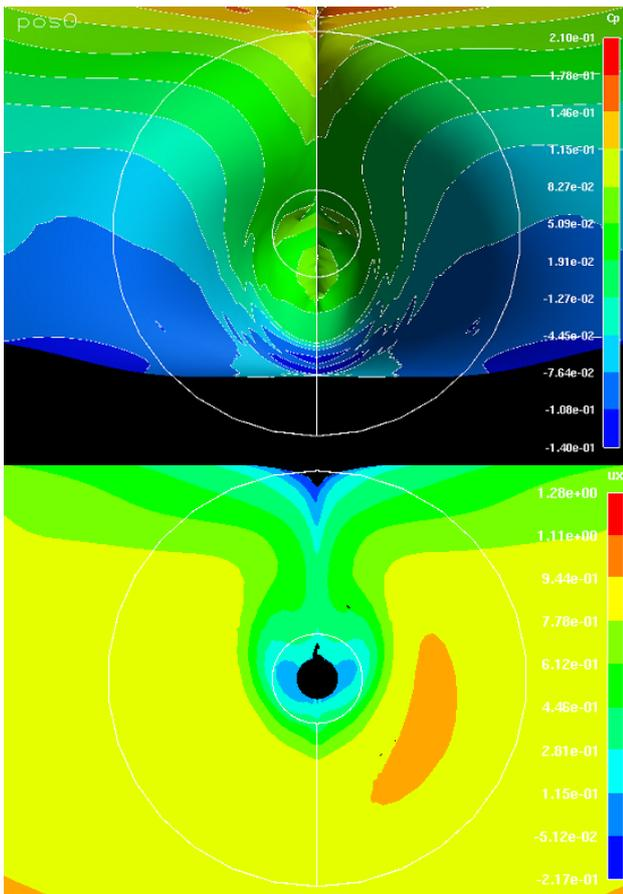
Figure 9: Pressure distribution on hull and total velocity just upstream the propeller for pos0 with LAP
