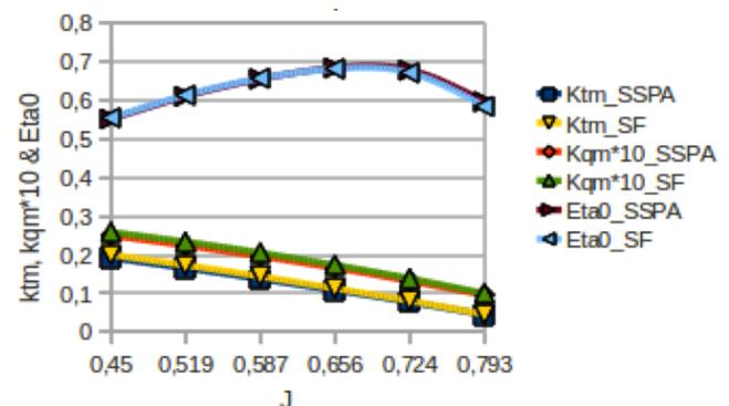
Figure 14: Comparing open water results for LAP using LL and experimental data
