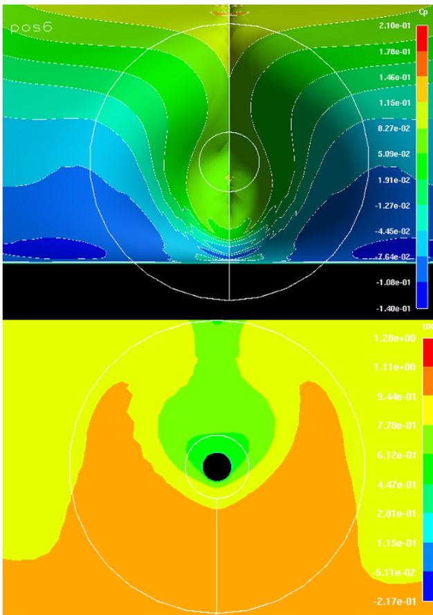
Figure 11: Pressure distribution on hull and axial velocity just upstream the propeller for pos6 with LAP
