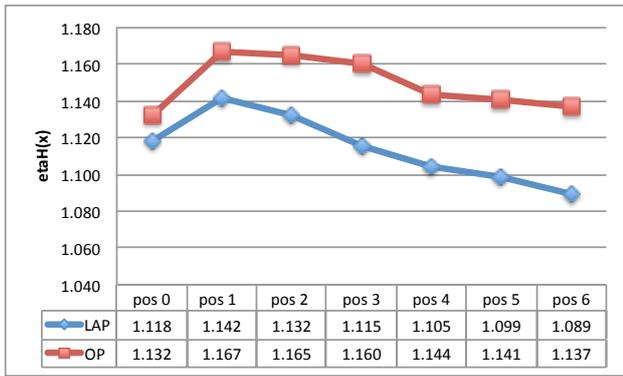
Figure 8: Variation of hull efficiency with propeller position; LAP vs OP
