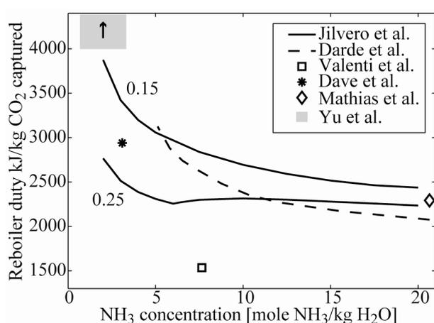
Figure 1. The specific reboiler duty when simulated with ammonia concentrations of 2-20 moles NH<sub>3</sub>/kg H<sub>2</sub>O and CO<sub>2</sub>-loadings of 0.15 and 0.25. The CO<sub>2</sub>-loading for the remaining sources: Darde et al. (0.33), Valenti et al. (0.25), Dave et al. (Unknown), Mathias et al. (0.36) and Yu et al. (0-0.6).
