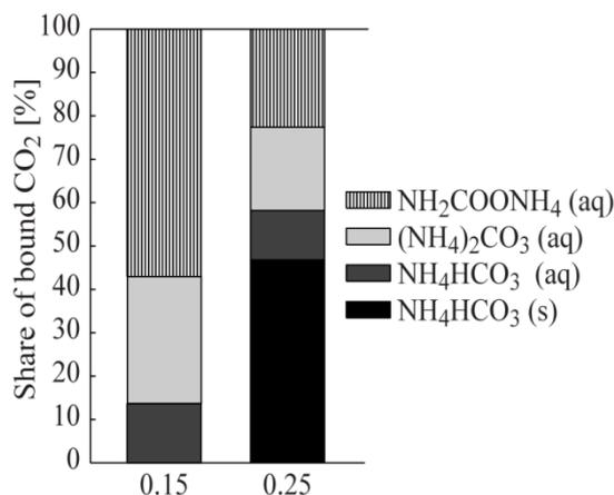
Figure 2. Distribution of how carbon dioxide is bound in the ammonia for CO<sub>2</sub>-loadings of 0.15 and 0.25. In these simulations an ammonia concentration of 15 moles NH<sub>3</sub>/kg H<sub>2</sub>O are applied. Simulations after Jilvero et al. [5].
