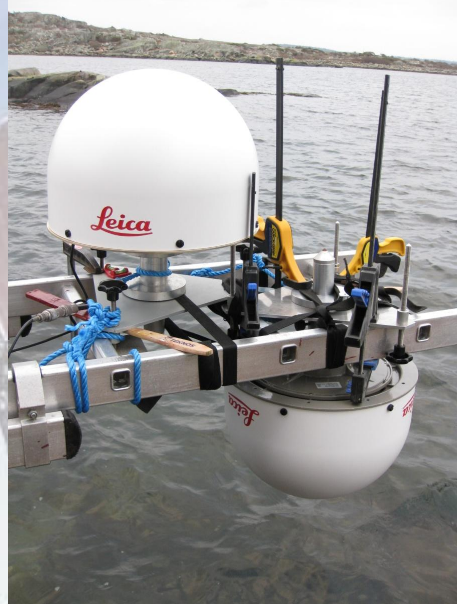
Figure 1. The experimental setup of the GNSS-based tide gauge at the Onsala Space Observatory (OSO).
