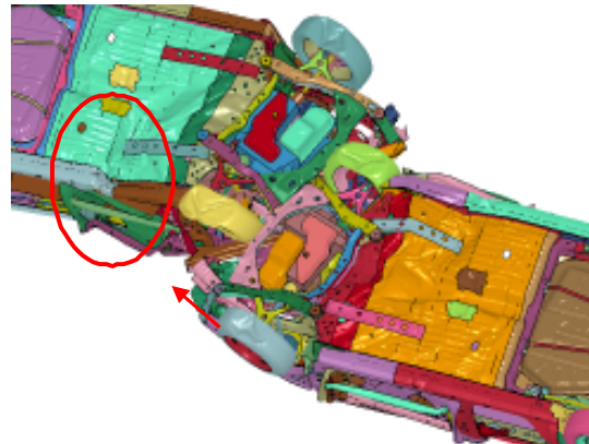
Figure 11: Buckling deformation of vehicle induced by moment force in B2S_H60V100
