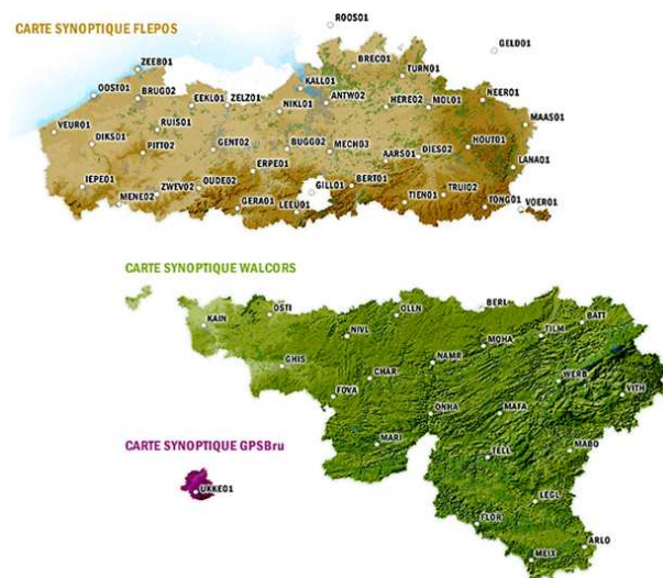
Figure 7.18: The local network developed in Belgium for real-time positioning.
