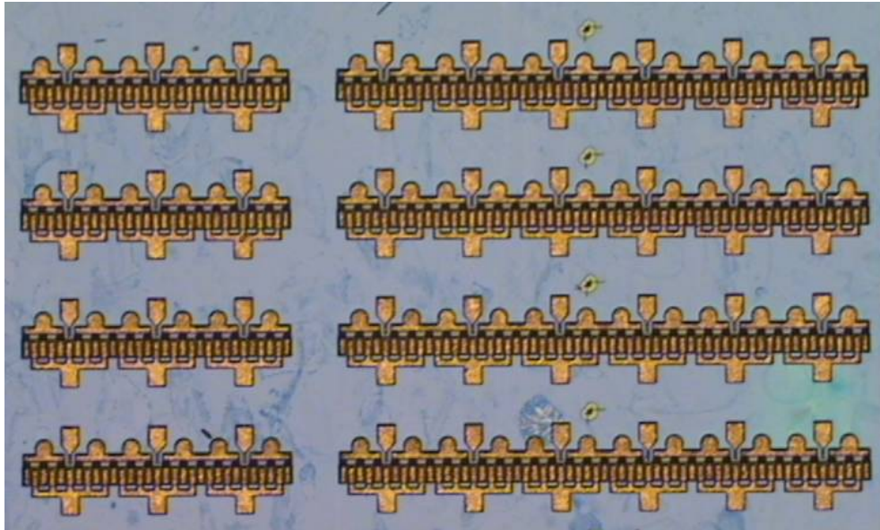
Figure 13. Via-hole grounded 3 mm and 6 mm SiC MESFETs using double-recessed field plated design. The SiC MESFET exhibited 7.8 W/mm at 3 GHz ( f_{\max} = 25 GHz).
