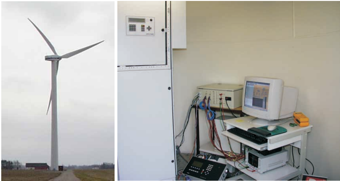
Fig. B.2. Jung wind turbine and the data acquisition computer.
