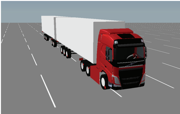
Figure 2: A long vehicle combination with eleven axles and 26 tyres.
