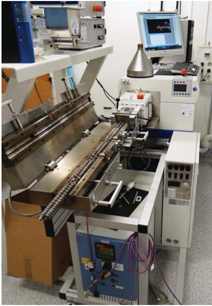
Figure 4. Brabender TSE 20/40 at RISE Borås, here with the barrel opened.
