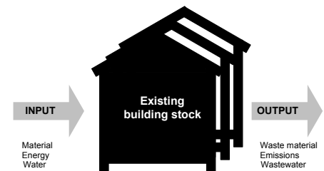
Figure 10.2. From the top-down approach, the existing stock is considered as a “black box”. Resource flows in the building stock: input of materials, energy, and water and output of waste materials, emissions, and waste water are considered.
