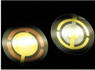
**Figure 1.3:** *Two quartz crystal resonators (QCMs). Image from [7] (CC-BY-3.0).*
