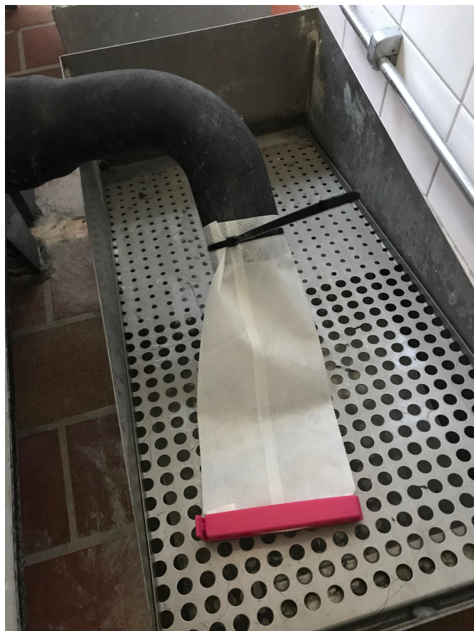
Figure 9. The picture shows the filter fastened on the end of the pipe with cable ties, and a plastic clip sealing the end.
