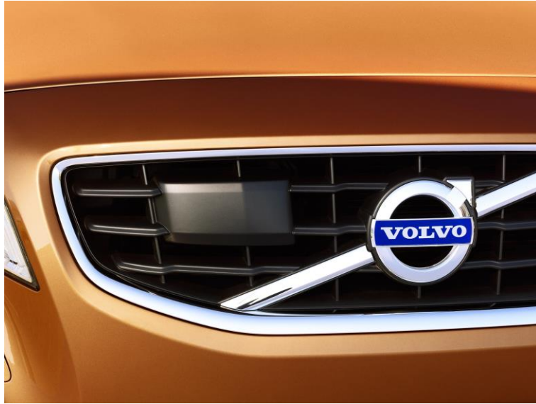
Figure 20: Placement of Volvo radar sensor
