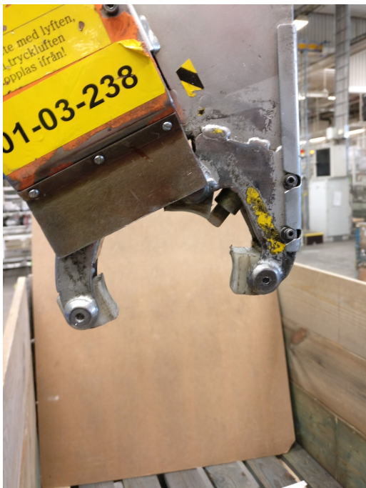
(a) Gripper and sensor triggering grip function seen in top right of gripper.
