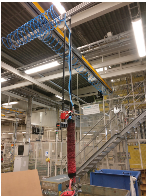
(a) Entire generator lifting device, showing overhead rails, attachment and gripping part.
