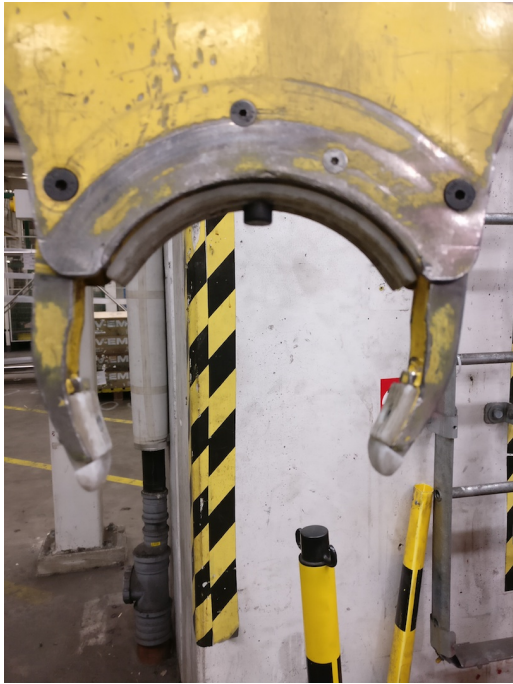
(a) Gripper with sensor triggering grip function seen in top of gripper.
