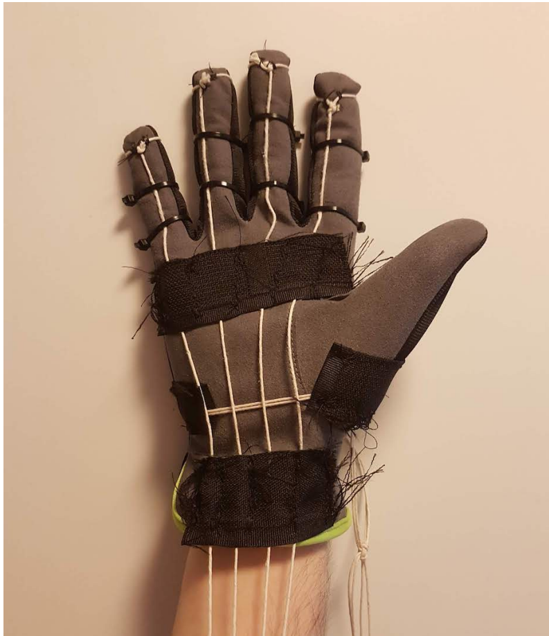
Figure 5.19: Prototype of actuated glove for verifying gripping function
