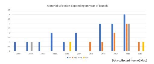
Figure 5.3: The figure illustrates a diagram which shows the material selection for the lower cover (of the door-panel) depending on which year it has been launched [53].
