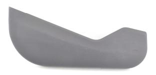
Figure 5.5: The lower cover for the car model BMW X1. It is designed as one part (only the lower cover) which is mounted to the panel carrier in a later stage. Copyright A2Mac1 [53].
