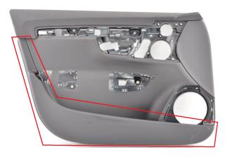
Figure 5.4: The lower cover for Volvo S90. It is designed as a merged part with the panel carrier and the lower cover. (The red marked part is the lower cover). Copyright A2Mac1 [53].
