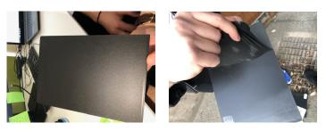
(a) Spray plastic applied to(b) Spray plastic during a test plate.(b) Spray plastic during process of removal.
