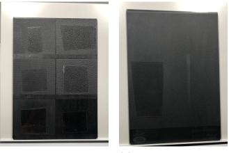
(a) Scratch & resistant tape applied to test plate 1.
