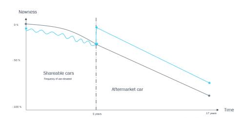
Figure 6.6: Visualizing the decrease in newness of baseline lower cover (starting from 0%) and of lower cover with a protective layer (starting from -10%).
