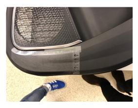
Figure 6.5: Scratch & wear resistant tape applied to a prototype lower cover.
