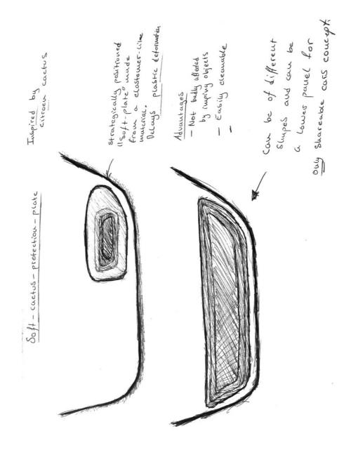
Figure G.7: Brainstorming idea 7, a design and material choice which delays plastic deformation.
