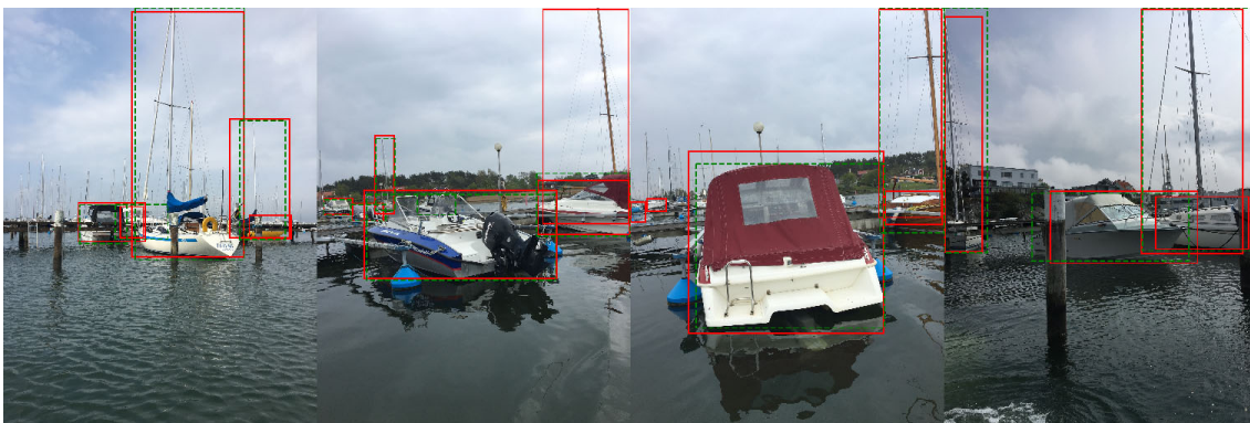
Figure 5.4: Images with duplicate detections of sailboats. Detections are shown as solid red rectangles and ground truth objects as dashed green rectangles.
