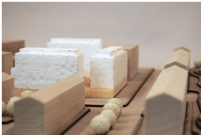
Figure 50. Opening a gap between building 2 and 3, and between building 3 and 4, provides some light and insight to the courtyard, while the translucent bottom floor keeps the courtyard private. What is visible in the physical model is that these gaps are actually quite narrow and might not have such a strong impact.
