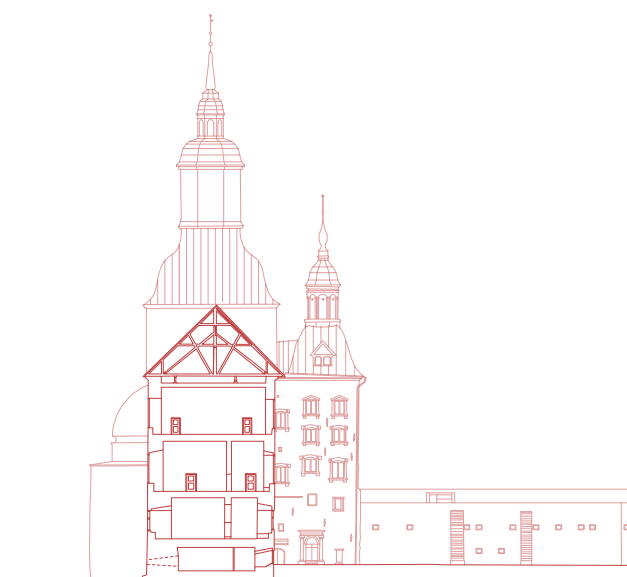
Figure 40. Section through one of the wings of the castle, 1:1000. The structure of the castle consists of thick stone walls, decreasing in width with each level, with wooden beams spanning between the walls and topped with a truss roof structure.
