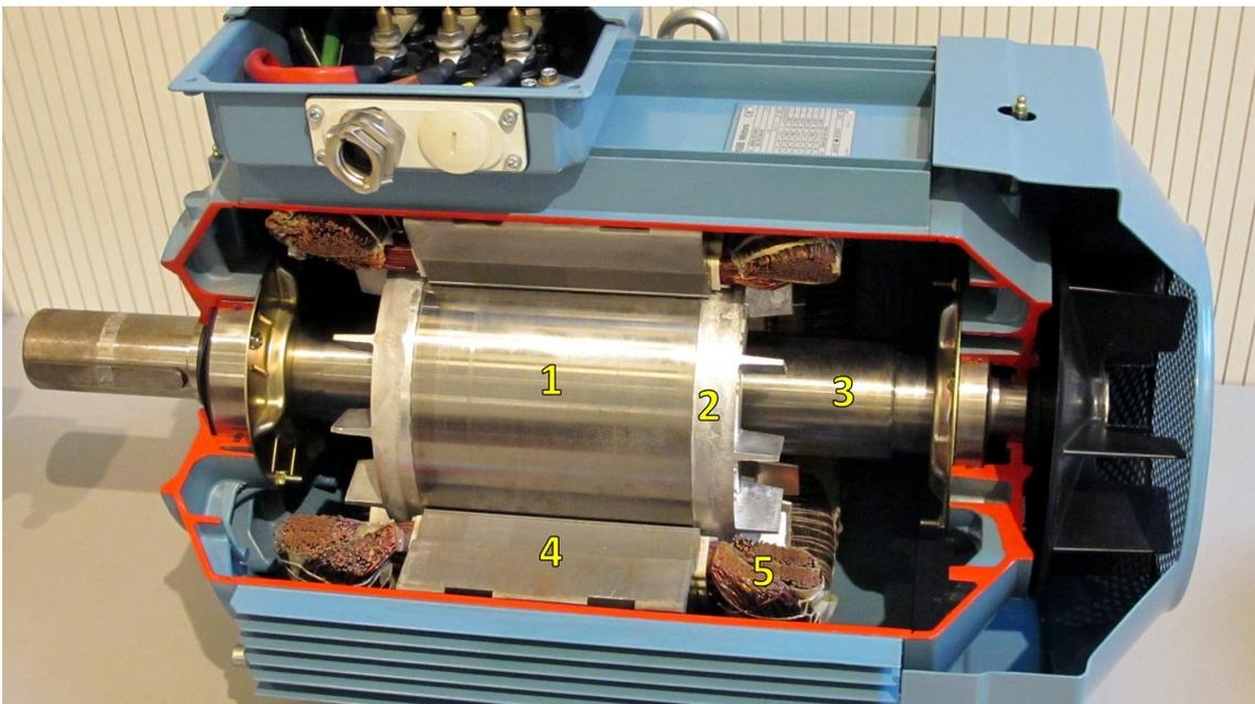
**Figure 2.1:** Cutaway model of an induction machine. 1) Rotor 2) Slip ring 3) Shaft 4) Active part of stator winding 5) Stator end winding. Adapted from [14]. Public domain.
