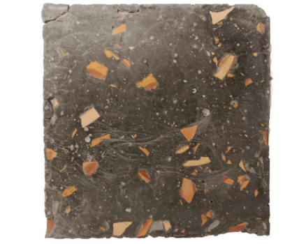
Roughly sanded with concrete sanding mashine
