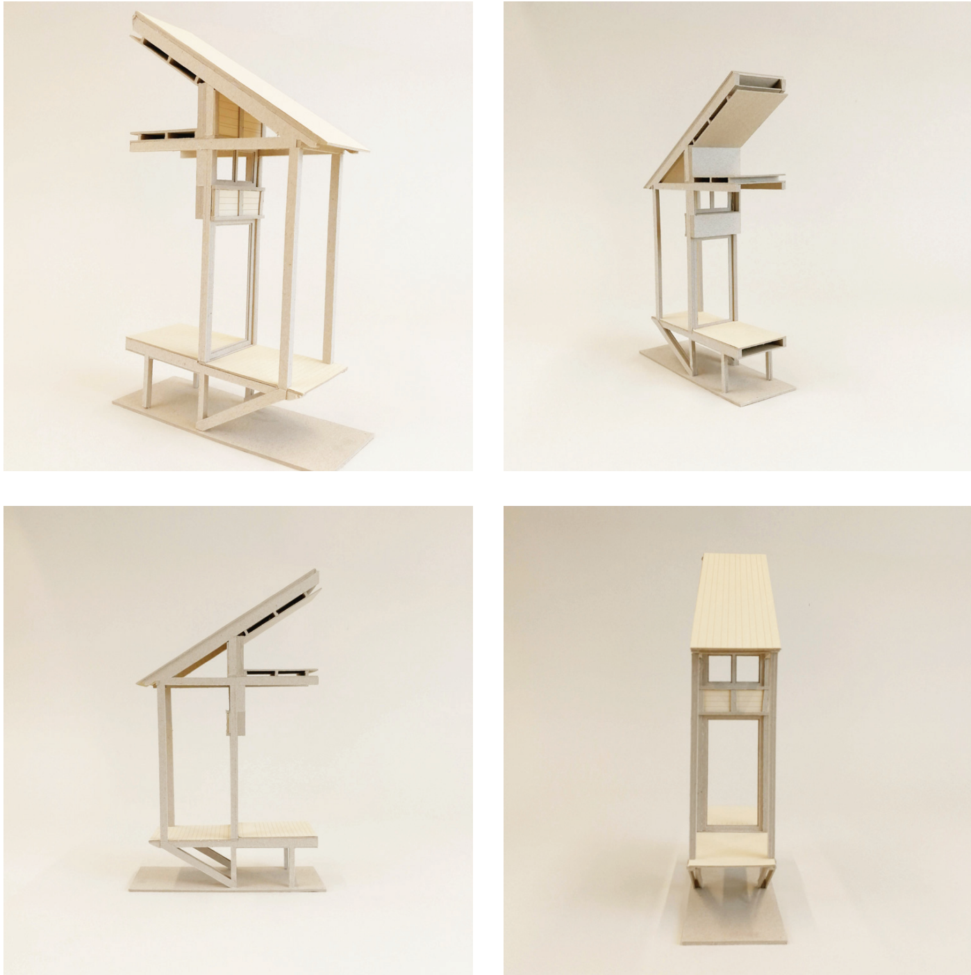
The detail model was made in scale 1:25 and cover a section of the bearing construction. The distance between the trusses and pillars is 1200 mm.
