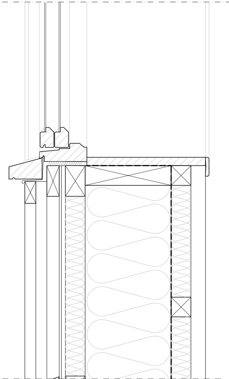
*Figure 109.* Detail showing window and sill, scale 1:5.
