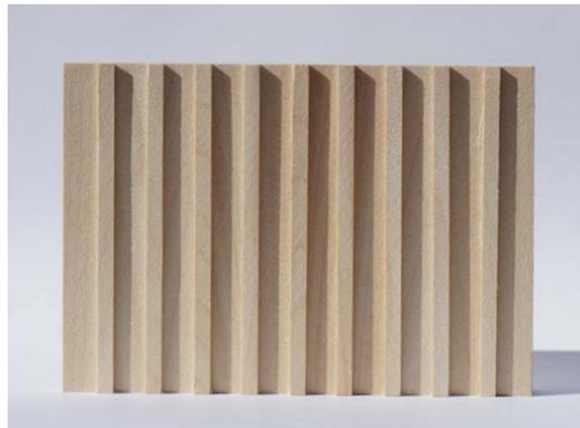
*Figure 14.* Board and batten.
