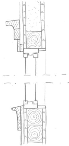
Figure 18. Principle of a timber frame wall.
