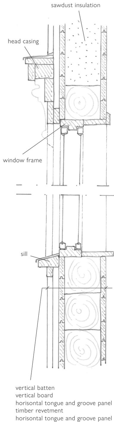
Figure 48. Detail sketch of the window
