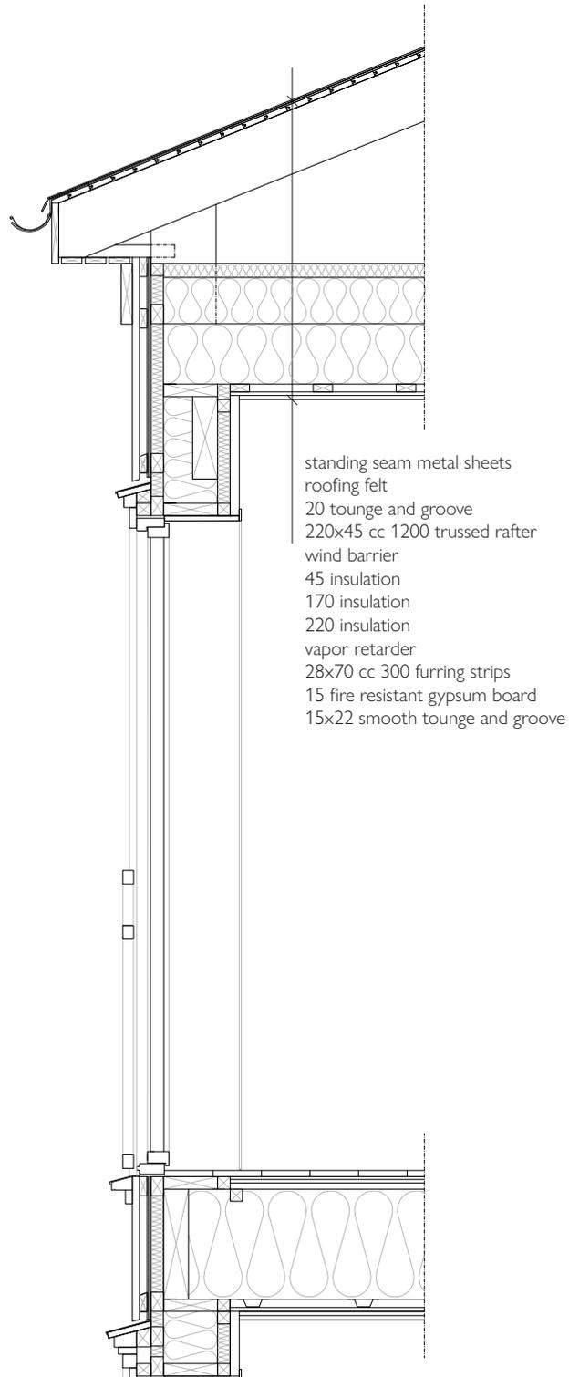
Figure 101. Section detail part 2, scale 1:25.
