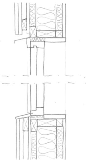
Figure 19. Principle of a balloon frame wall.
