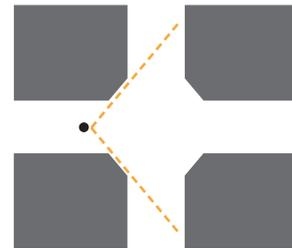
Figure 35. Sightlines with chamfered corners.
