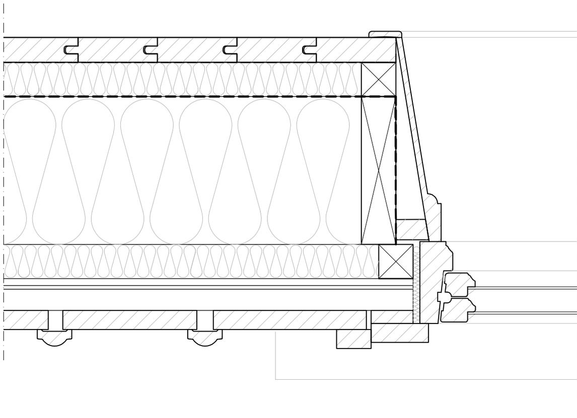
Figure 111. Detail showing window niche, scale 1:5.
