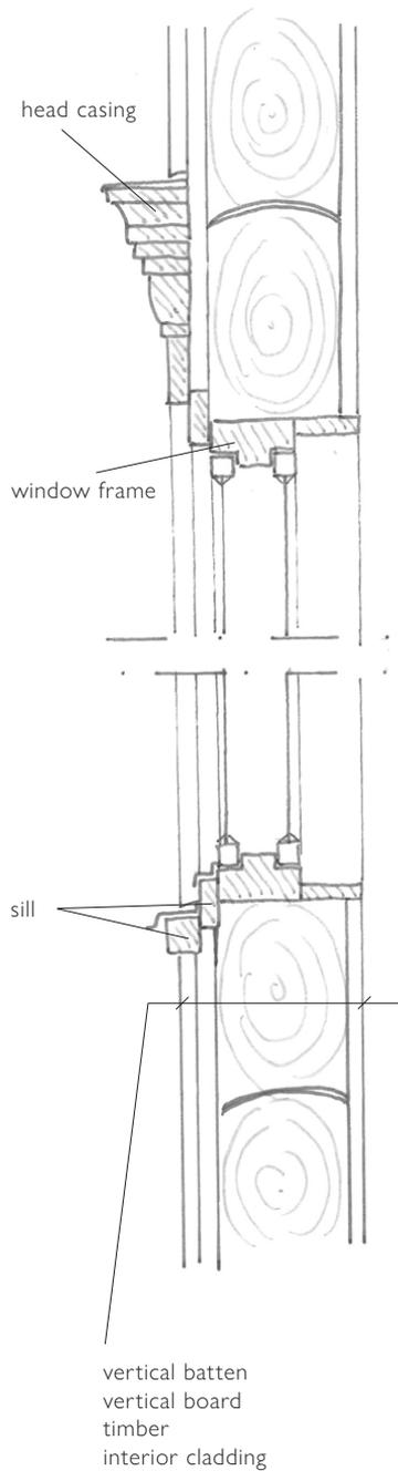
Figure 45. Detail sketch of the window.
