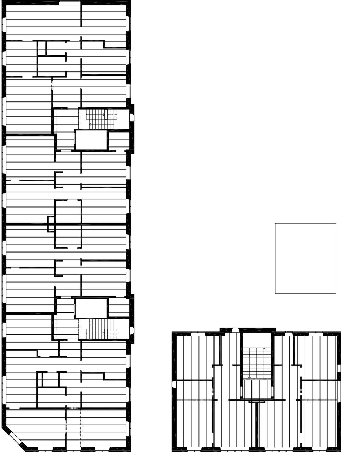
Figure 113. Plan for beams, scale 1:200. Beams showed on second story.
