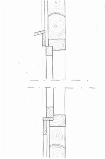
Figure 17. Principle of a timber wall.
