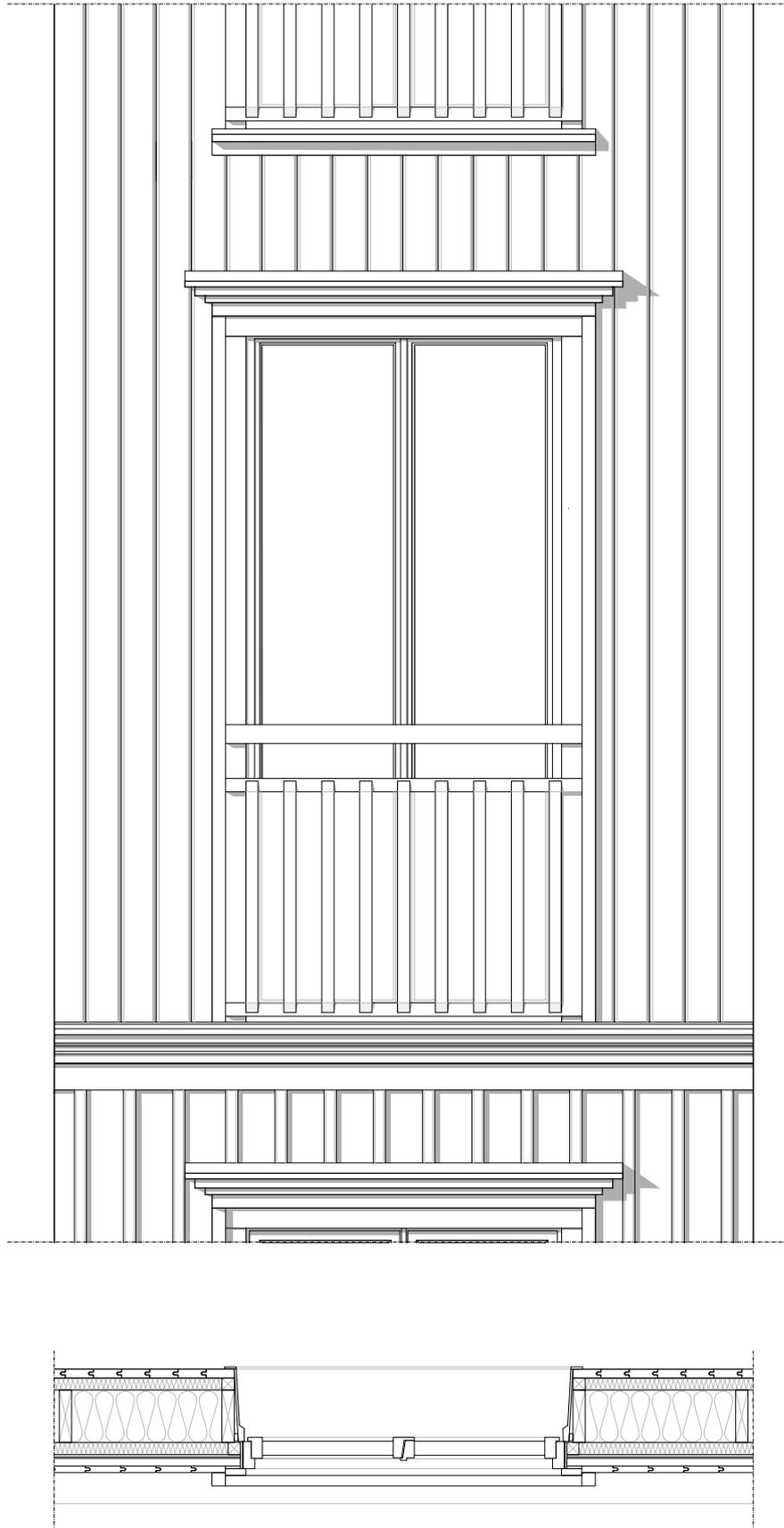
Figure 104. French balcony detail, scale 1:25.
