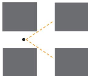
Figure 34. Sightlines without chamfered corners.
