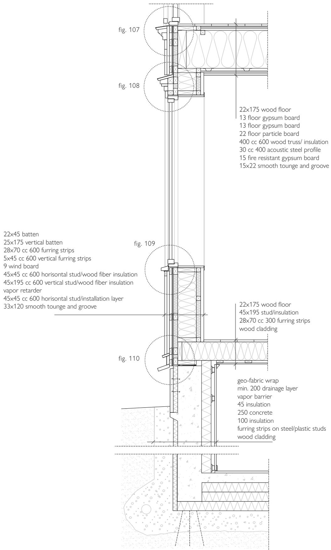
Figure 105. Section detail part 1, scale 1:25.
