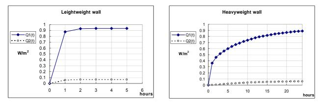
Figure A4.2 Thermal response of the lightweight and the heavyweight wall on internal radiative heat source
