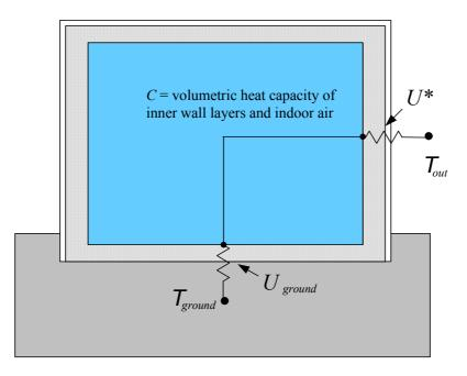
Figure A2.1 The model for the determination of the thermal time.
