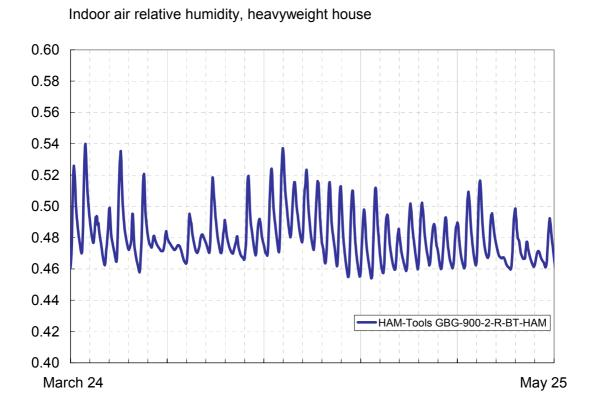
Figure 13 Indoor air relative humidity for the Case 2R-BT-HAM.
