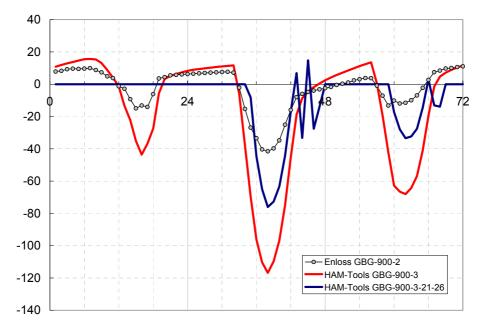
Figure 12 Hourly heating / cooling energy demands for Case 3 with two different heating / cooling set point temperatures: 21/21 °C and 21/26 °C (GBG-900). Enloss results for Case 2 are given as the reference.
