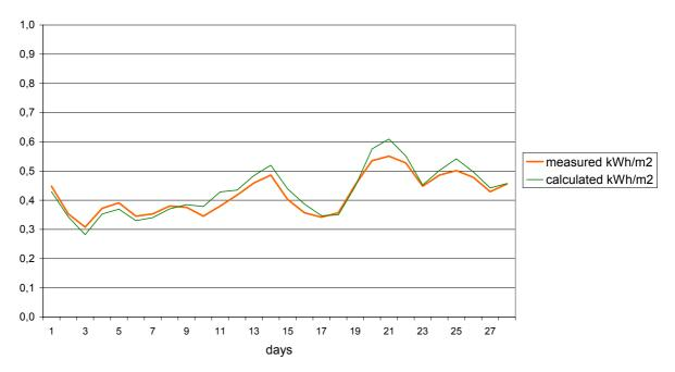
Figure A7.4 Measured and calculated energy consumption, daily values, Feb 2002.
