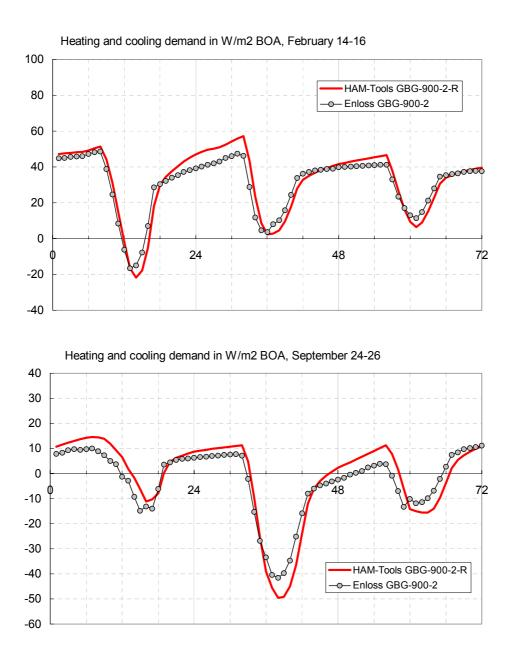
Figure 6: Hourly heating / cooling energy demands for the test cases GBG-900-2.
