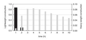
Figure 4. Weighting factors according to the DTN method (Eq. 12) for the lightweight (black bars) and the heavyweight construction (gray bars). The number of backward steps are 3 and 65 respectively.
