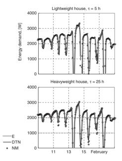
Figure 8. Instantaneous values of the heating energy demand for the standard-test house with ventilation and radiative solar gains, calculated by the three different methods.
