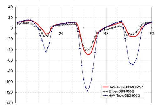
Figure 10 Hourly heating / cooling energy demands for Case 3 (GBG-900). Enloss results for Case 2 and HAM-Tools results for Case 2-R are given as the references.
