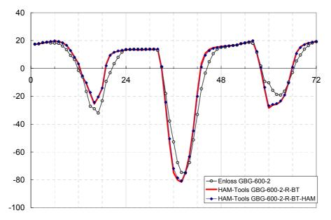
Figure 14 Hourly heating / cooling energy demands for Case GBG-600-2-R when the moisture load is taken into account. The HAM-Tools solution with moisture calculations is denoted with 2-R-BT-HAM. The HAM-Tools solution without moisture load is 2-R-BT. The BESTEST model for the heat transfer coefficients is used for the HAM-Tools solutions. Enloss results for Case GBG-600-2 are given as the reference.
