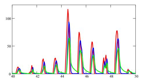
Figure A4.4 The effect of the solar radiation as the radiative heat source, calculated by the solar weighting factors: for the lightweight house (blue line) and for the heavyweight one (light green), in  $W/m^2$  of the floor area. The total incoming radiation is shown with the red line, from the Gothenburg climate data file.
