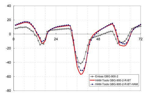
Figure 15 Hourly heating / cooling energy demands for Case GBG-900-2-R when the moisture load is taken into account. The HAM-Tools solution with moisture calculations is denoted with 2-R-BT-HAM. The HAM-Tools solution without moisture load is 2-R-BT. The BESTEST model for the heat transfer coefficients is used for the HAM-Tools solutions. Enloss results for Case GBG-900-2 are given as the reference.
