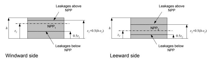
Leakages on the walls at the side of the windward wall, to be called here "the side walls", are positioned in the middle of the wall height:
