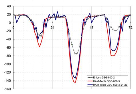
Figure 11 Hourly heating / cooling energy demands for Case 3 with two different heating / cooling set point temperatures:  $21/21 \,^{\circ}$ C and  $21/26 \,^{\circ}$ C (GBG-600). Enloss results for Case 2 are given as the reference.
