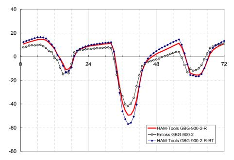
Figure 8 Hourly heating / cooling energy demands for Case GBG-900-2-R. Comparison between the Enloss and the BESTEST model (2-R-BT) for the heat transfer coefficients. Enloss results for Case GBG-600-2 are given as the reference.
