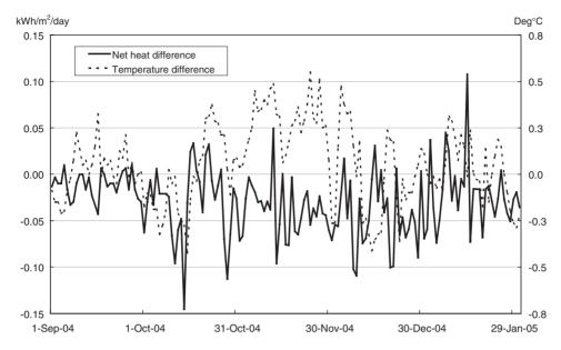
Figure 2. Comparison of differences the net energy use for space heating and indoor air temperatures in the test and the reference building (test – reference).
