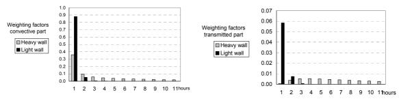
Figure A4.3 Thermal response factors (weighting factors) for solar radiation as the internal radiative heat source
