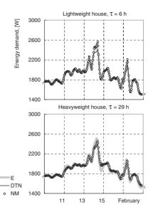
Figure 6. Instantaneous values of the heating energy demand for the standard-test house, calculated by the three different methods. No ventilation or solar radiation is introduced.
