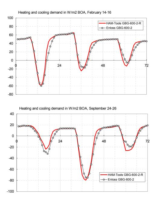
Figure 5: Hourly heating / cooling energy demands for the test cases GBG-600-2.
