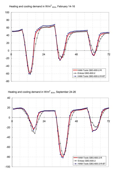
Figure 7 Hourly heating / cooling energy demands for Case GBG-600-2-R. Comparison between the Enloss and the BESTEST model (2-R-BT) for the heat transfer coefficients. Enloss results for Case GBG-600-2 are given as the reference.
