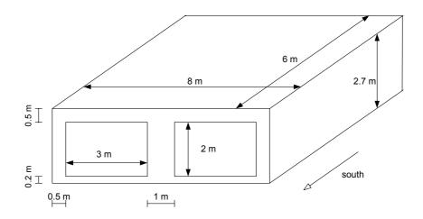
Figure 2 Geometry specification for the test building
