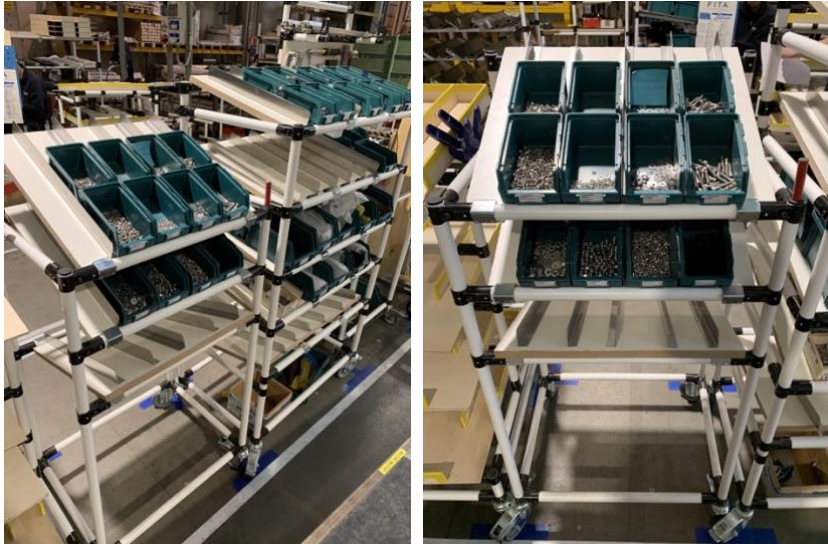
Figure 50, Physical representation of the double-bin method
