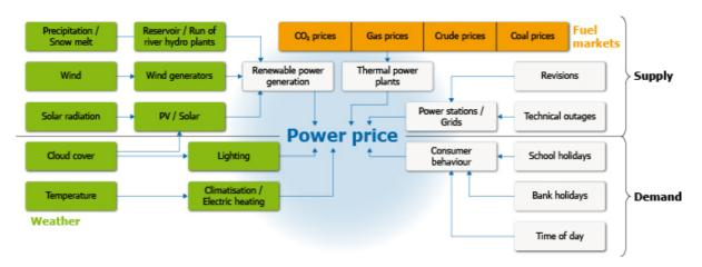
Figure 1: Factors influencing the spot price of electricity. Source: RWE AG.
