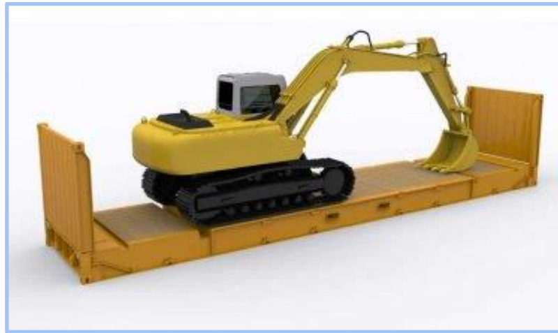
Figure 3-4: Example of a flat-rack with H&H cargo (Gungor, 2018).
