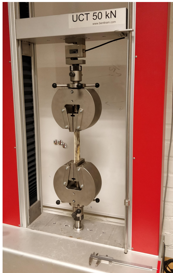
Figure 3.5: The test set up with a wide specimen in the TRAM UTC 50kN.
