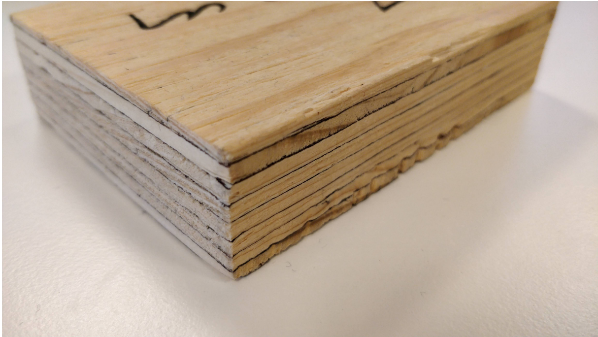
Figure 2.5: Laminated Veneer Lumber, LVL. Observe the ply lay-up that is the same as in Figure 2.6, although the bottom half-ply is missing in this picture.
