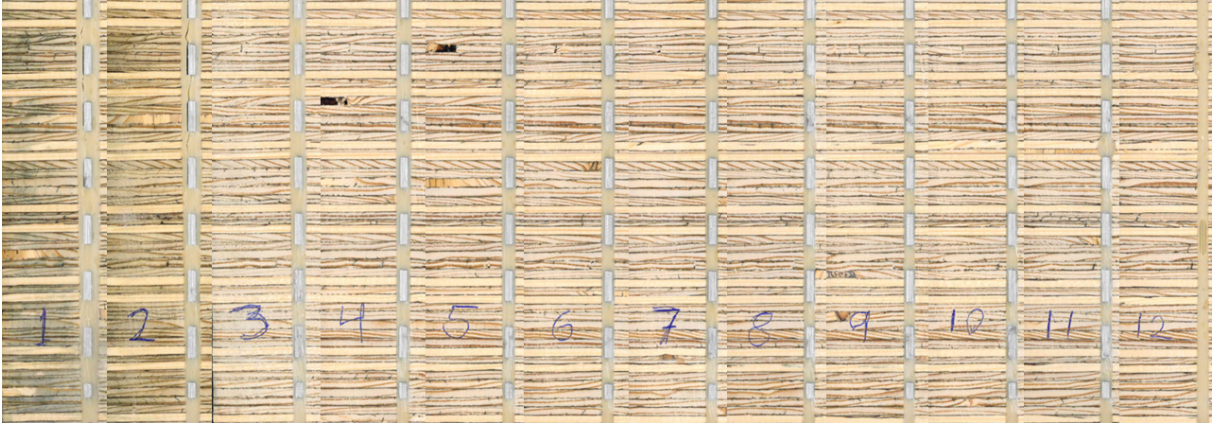
Figure 3.13: Sample 4, main side cut scans. Each cut is 30 mm apart. Sample 4 has been tested for fatigue at more than 30 000 cycles, where the load is unknown to us.
