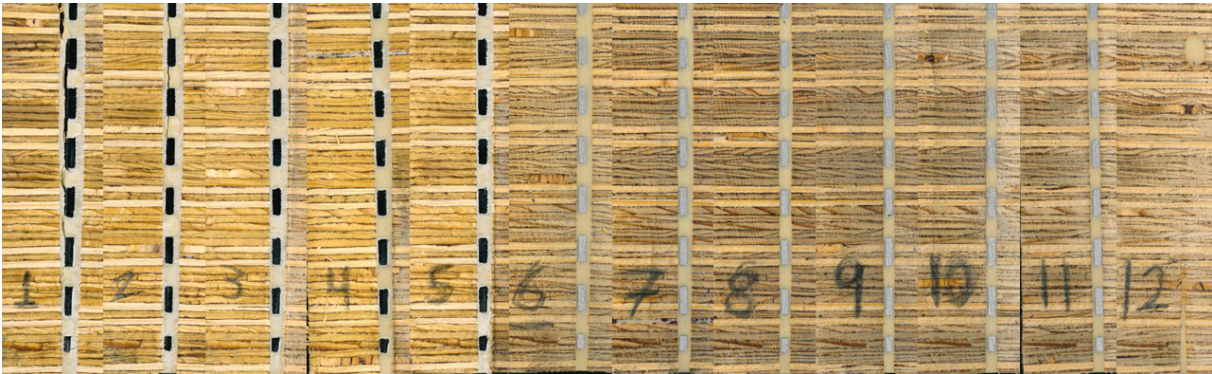
Figure 3.15: Sample 5, main side cut scans. Each cut is 30 mm apart. Sample 5 has been tested in pure tension and broke at 269 kN.
