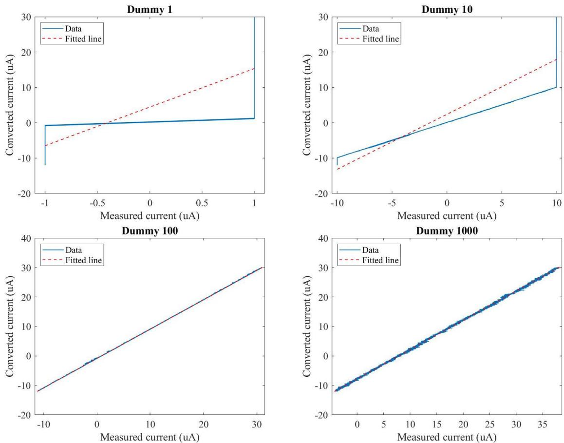
Figure 17, curves of the measured current compared to converted current from the calibration of Rodeostat via a dummy cell.
