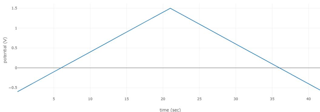
Figure 4, CV made on dummy cell between  $-0.6\text{ V}$  and  $1.5\text{ V}$  with the scan rate of  $0.1\text{ V/s}$ . Graph show the change in potential over time.
