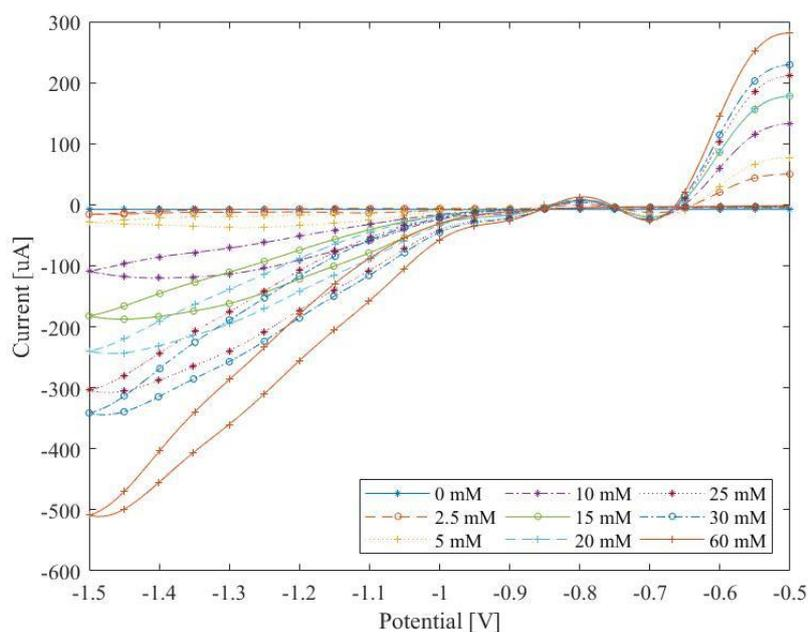
Figure 18, example of cyclic voltammogram measurement from one SPCE-AuNP with increasing concentration of lactic acid in 0.1 M KCl (tap water)
