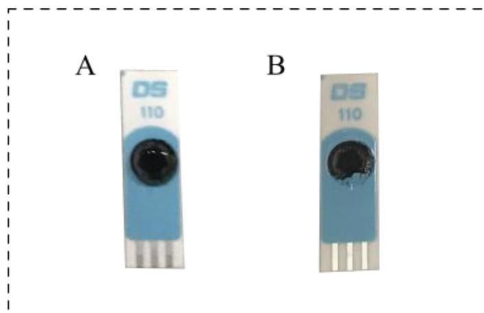
Figure 15, A: picture of SPCE-AuNP after addition of MIP solution, B: picture of the modified electrode after drying.
