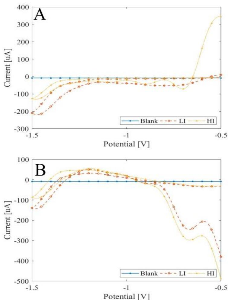
Figure 21, cyclic voltammogram of sweat samples on A: SPCE-AuNP and B: modified SPCE-AuNP.
