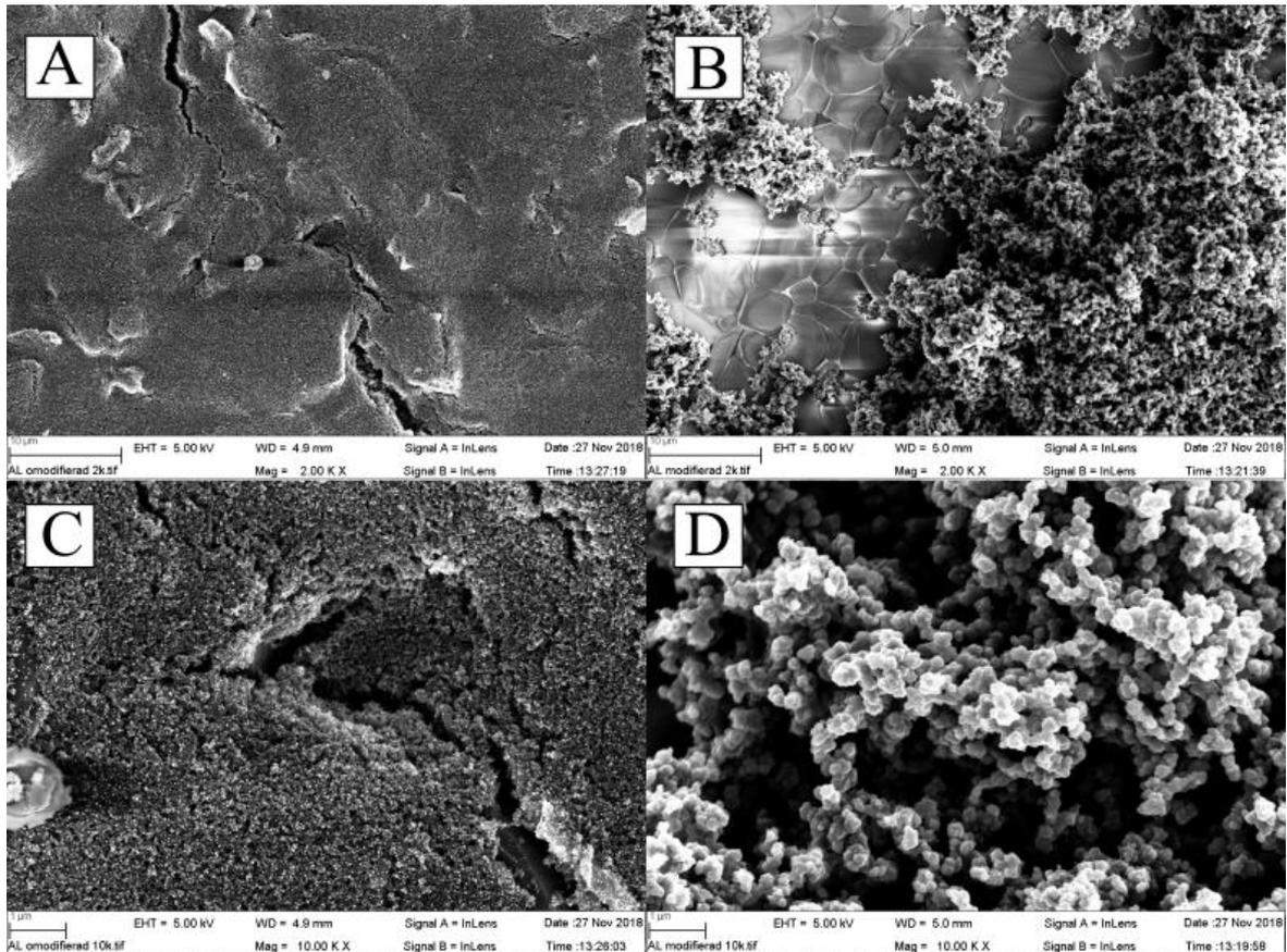
Figure 16, SEM picture of the SPCE-AuNP without and with modification. A: SPCE-AuNP at 2000 times magnification, B: modified SPCE-AuNP at 2000 times magnification, C: SPCE-AuNP at 10000 times magnification and D: modified SPCE-AuNP at 10000 times magnification.
