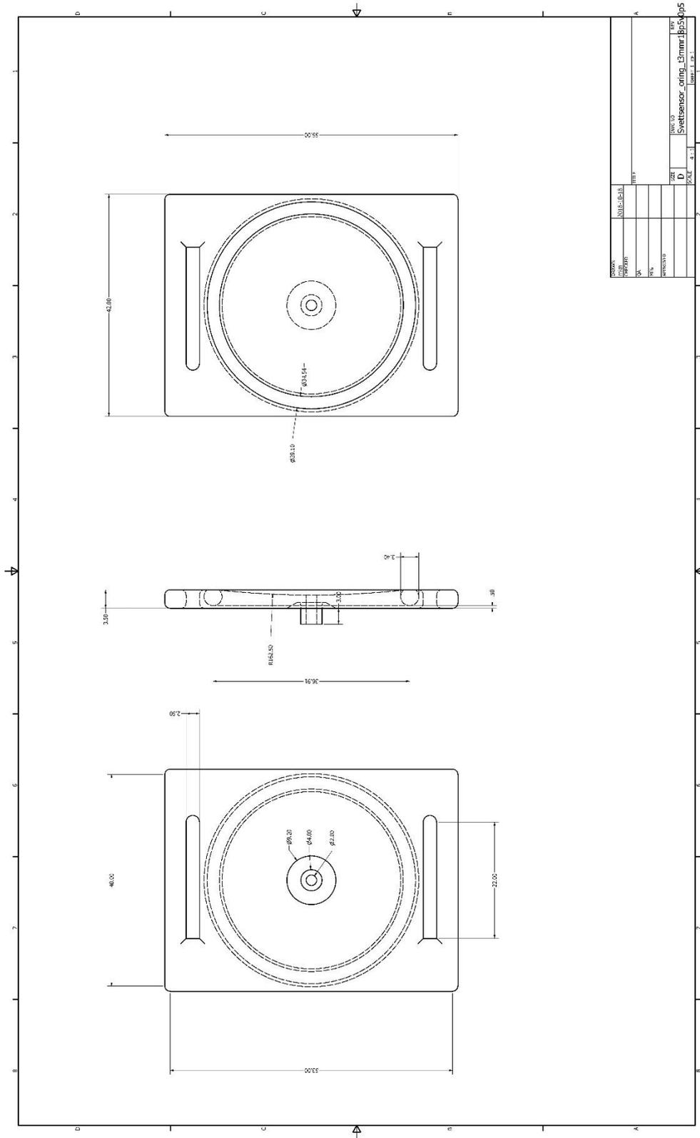
Figure B1, design of sweat collector with place for an O-ring.
