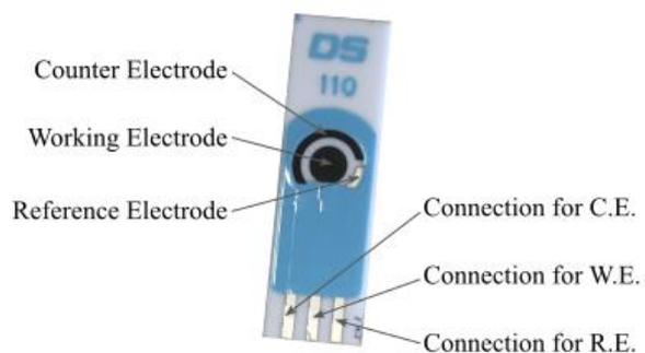
Figure 5, picture of a screen-printed carbon electrode with gold nanoparticles from DropSens with the different electrodes and connections are pointed out.
