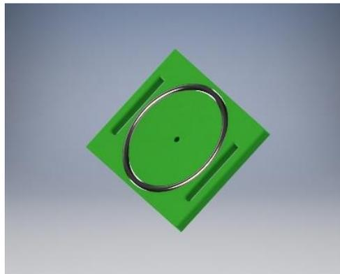
*Figure 8, model of sweat collector with O-ring.*
