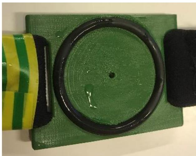
Figure 11, sweat collector ver.2 after test. A small sweat accumulation can be seen on the collector.
