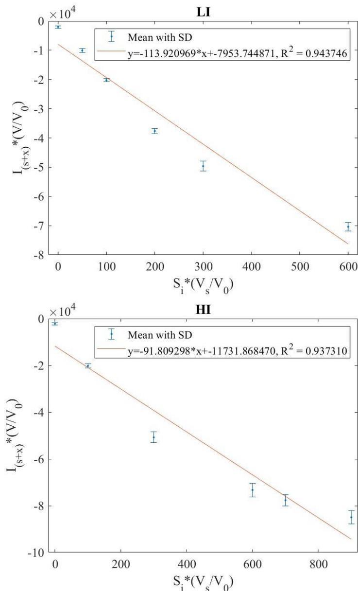
Figure 12, graphs from standard addition for sweat collected at low (LI) and high (HI) intensity.
