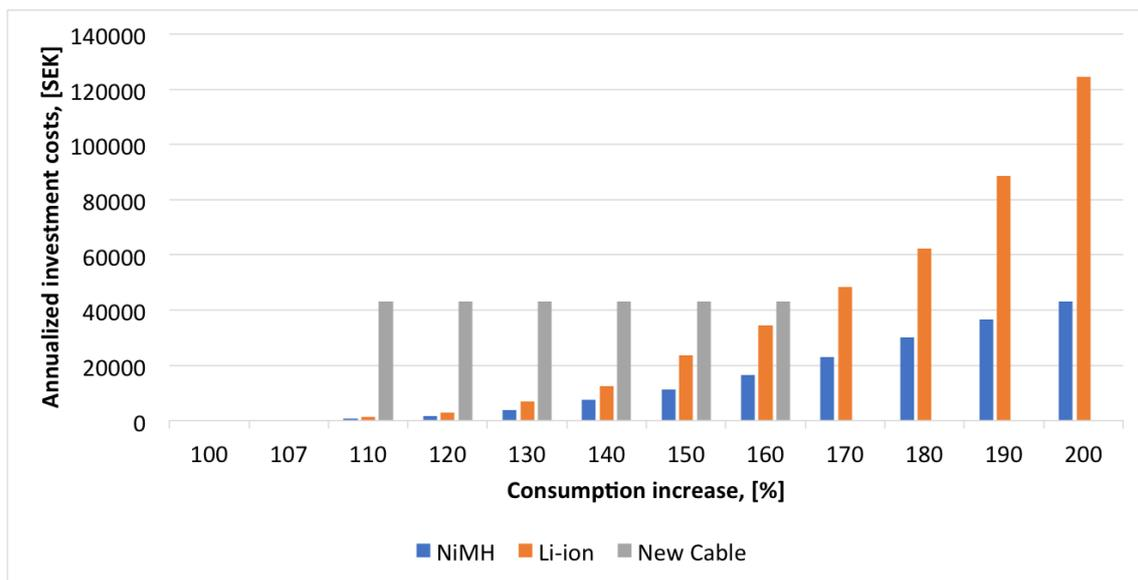
**Figure 5.10:** The annualized investment cost in SEK for each solution and the levels of demanded increase. The 100% represents a peak demand of 13.6 kW.
