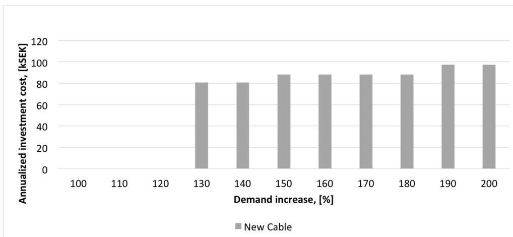
**Figure 5.4:** The annualized investment costs in SEK for the cable solutions and the levels of increased demand. The 100% represents a peak demand of 1257 kW.
