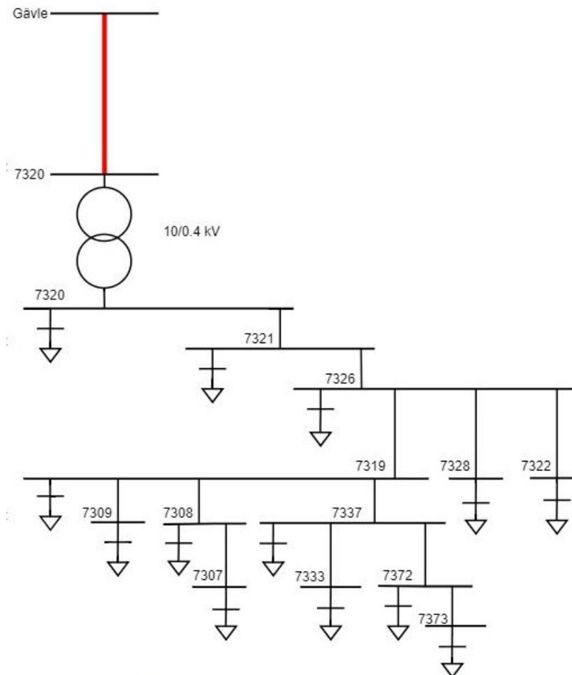
**Figure 4.1:** Configuration of the grid in Furuvik. The red line represents the overhead line which needs reinforcement in order to provide the demanded power to Furuvik.
