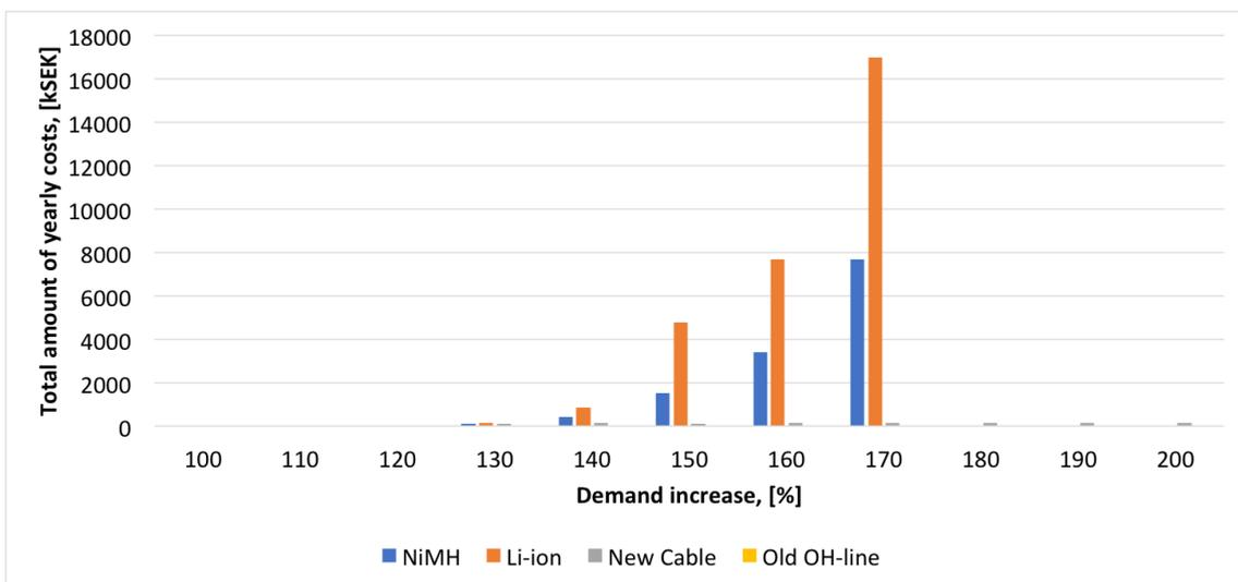
**Figure 5.6:** The total yearly costs for all solutions in SEK and the levels of demanded increase. In the total costs losses and investment costs are included. The 100% represents a peak demand of 1257 kW.
