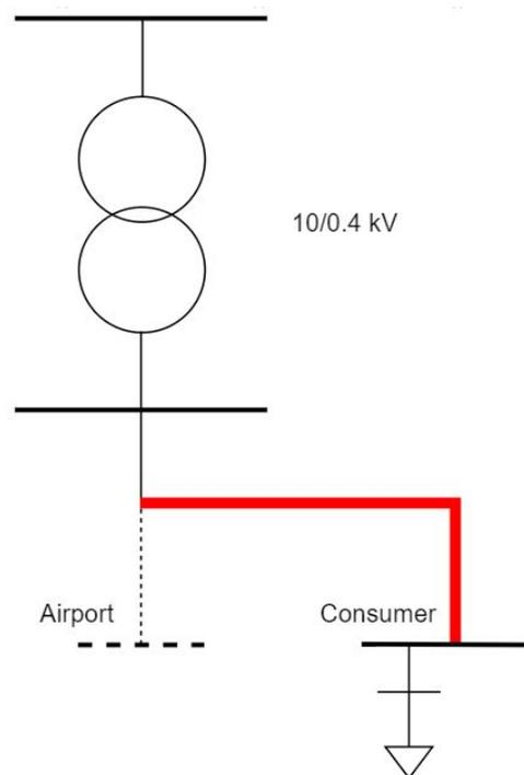
**Figure 4.5:** Configuration of the grid at Kalmar-Öland Airport. The red line represents the cable which needs reinforcement in order to provide the demanded power to the customer.
