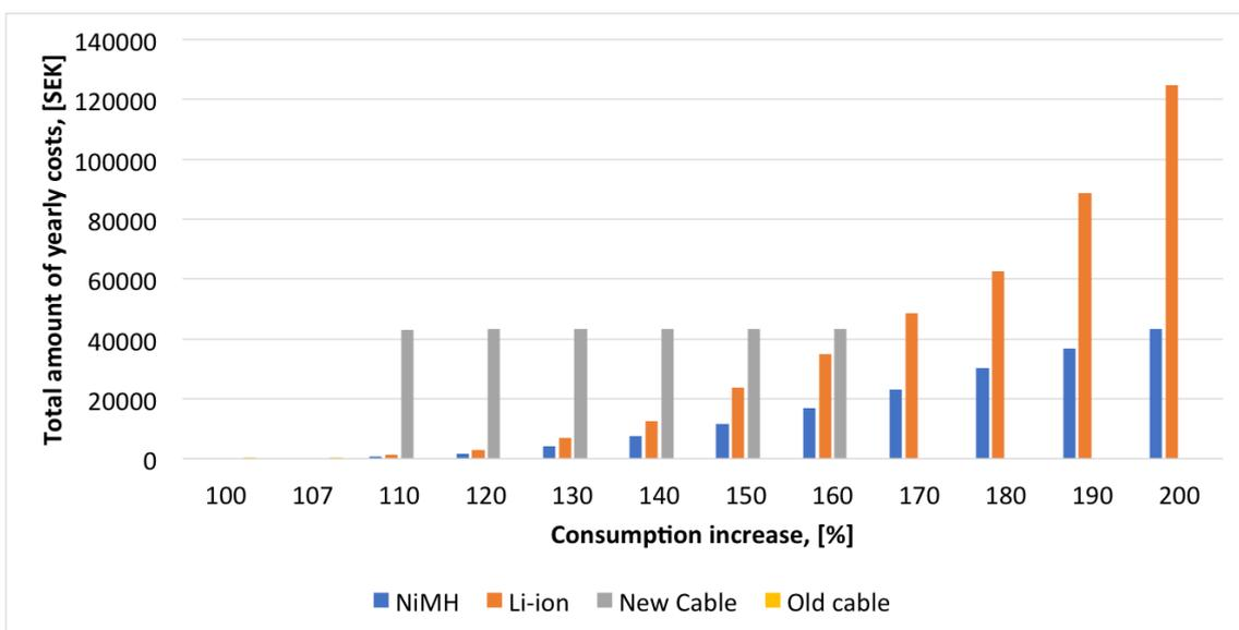
**Figure 5.12:** The total yearly cost (investment and losses) in SEK for each solution and the levels of demanded increase. The 100% represents a peak demand of 13.6 kW.
