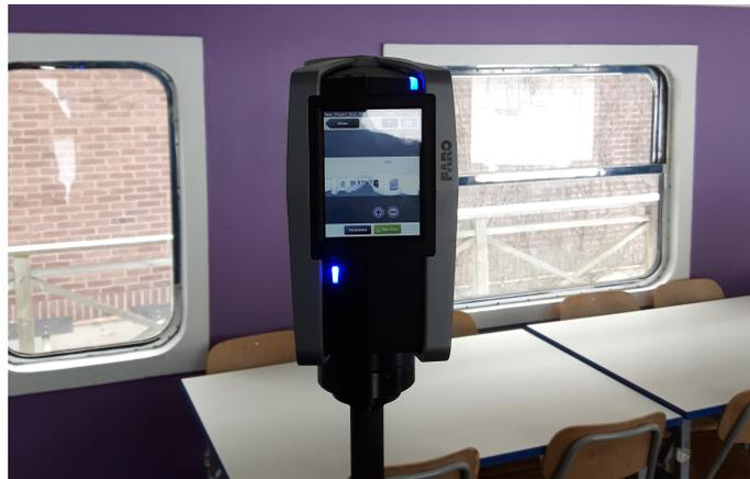
**Figure 3.7:** Side view of FARO Focus 3D scanner standing inside train carriage. The scanners touch display is facing the camera.
