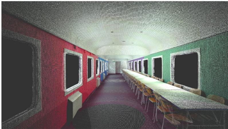
(b) From inside of the train carriage used for measurements. Note that details such as the arcs in the ceiling have been successfully depicted.
