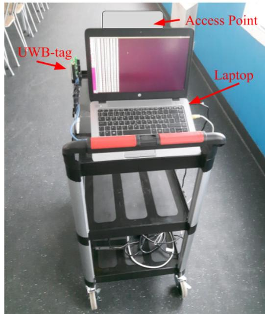
**Figure 3.4:** Cart used for measurements, UWB positioning tag (left), laptop used for measurements (center) and access point (behind laptop screen).
