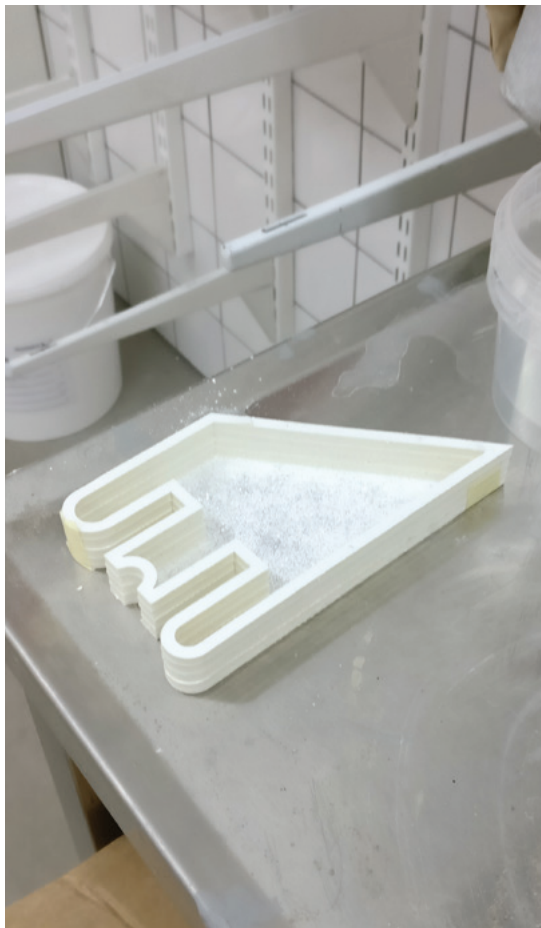
Fig. 68. Making of facade elements, CNC-cut formwork out of foamcore cardboard.
