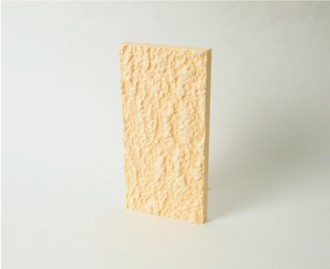
Fig. 70. CNC-milled Styrofoam (XPS).
