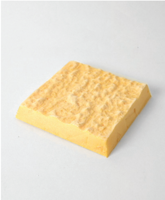
Fig. 47. CNC-milled Styrofoam positive. (Author's own copyright.)
