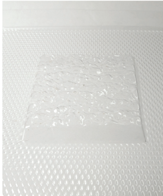
Fig. 48. Vacuum-formed PET negative. (Author's own copyright.)
