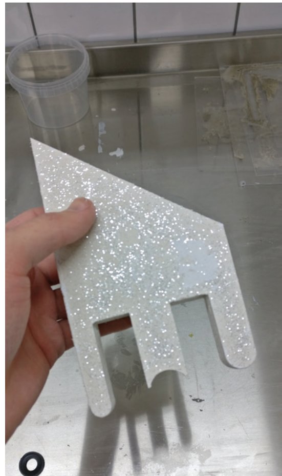
Fig. 69. Spray-glued glitter in the formwork transfers onto the element.
