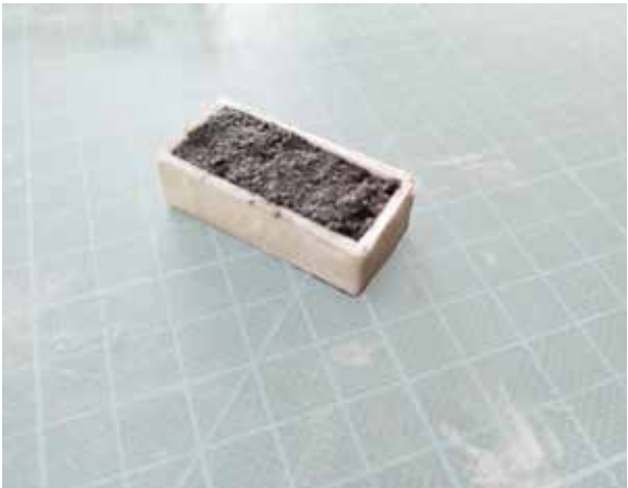
1. Molding Bricks, 75% sand, 25 % blue clay.
