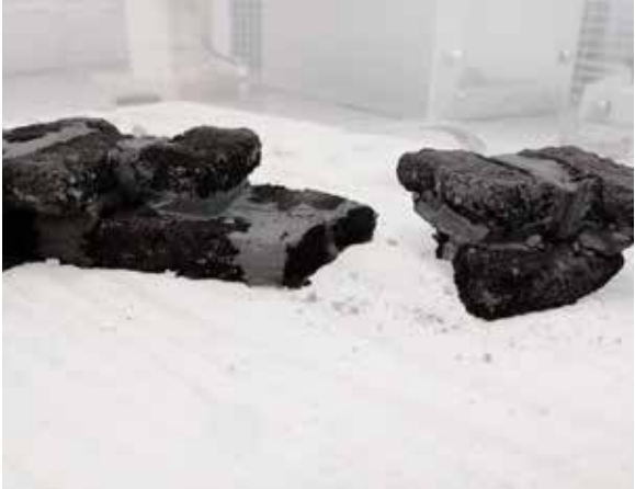
2. Soaked bricks appeared to be very fragile and ruptures emerged in the structure, when moving it before drying.
