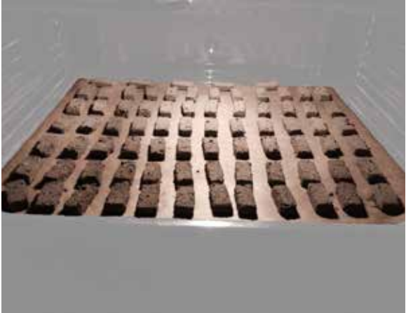
2. Baking bricks in oven, 105° 1 hr. (to simulate sun drying)
