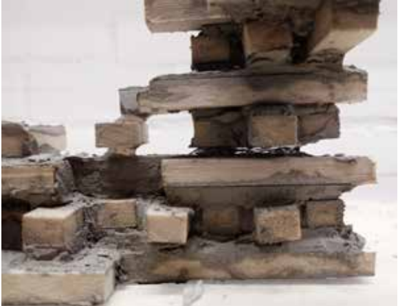
5. Critical areas were reinforced with glue.
