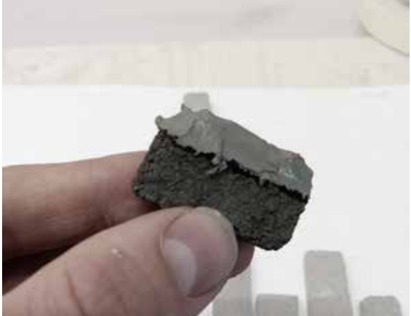
4. Depending on the situation, mortar was applied either on the brick or on the course below.
