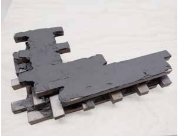
4. Cracks were filled, and a layer of mortar was applied on top of each course for better cohesion
