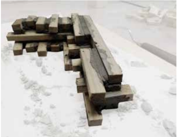
3. Cracks appeared after drying
