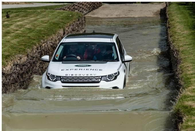
Figure 1.1.1: A car wading through deep water at a test facility. Figure obtained from [7], published with permission.
