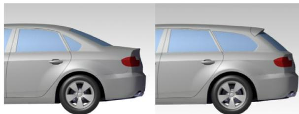
(b) *Notchback rear end (left) and estate back rear end (right).*
