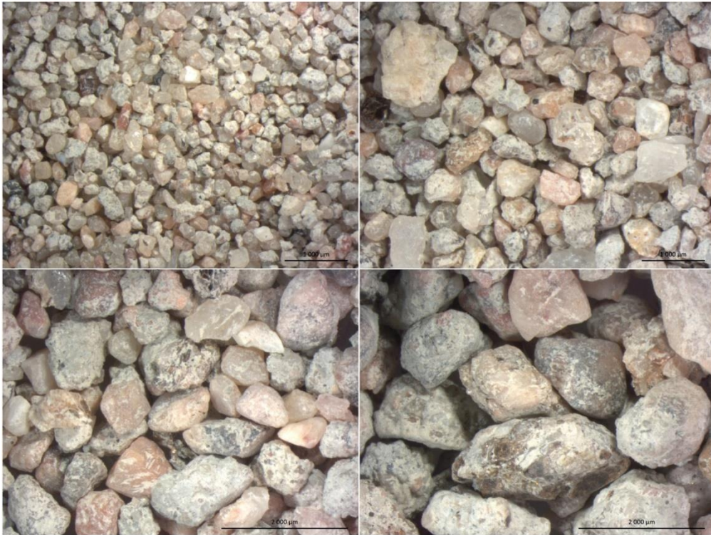
Image 5. Washed aggregates from the thermal treated concrete. In the top left corner is the fraction 0.125-0.5 mm and next to it is the fraction 0.5-1 mm. Down in the left corner is the 1-2 mm fraction, and next to it is the 2-4 mm fraction.
