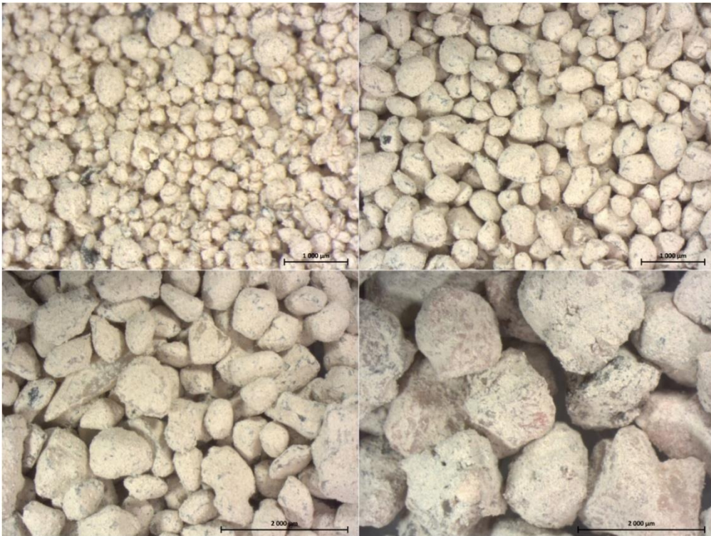
Image 6. Washed aggregates from the non-thermal concrete. In the top right-hand corner is the fraction 0.125-0.5 mm and next to it is the fraction 0.5-1 mm. Down in the left corner is the 1-2 mm fraction, and next to it is the 2-4 mm fraction.
