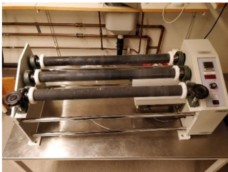
Image 3. The ball mill that, together with the metallic containers (Image 2), was used to mill the concrete.
