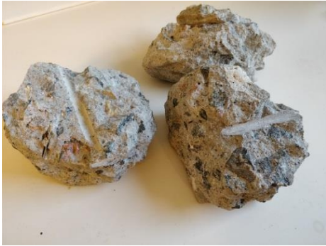
Image 1. The concrete that was used in the study. The reinforcing bars had been removed before the concrete was received.
