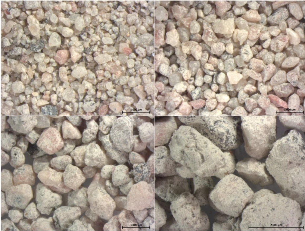
Image 4. Non-washed aggregates from the thermal treated concrete. In the top left corner is the fraction 0.125-0.5 mm and next to it is the fraction 0.5-1 mm. Down in the left corner is the 1-2 mm fraction, and next to it the 2-4 mm fraction.
