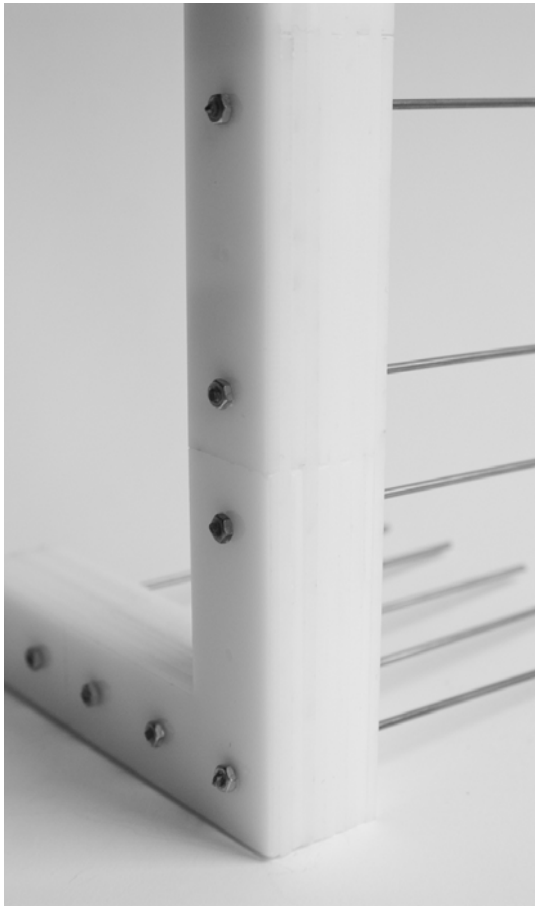
Scale 1:10 detail model. Early study of a different construction technique where the walls are made up of 6 different sized pieces that overlap.
