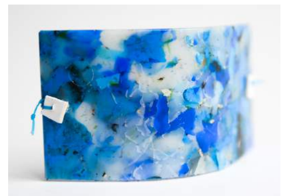
Bending the plastic sample using a tension wire The result - the plastic cracks and the grain boundaries imply weakness
