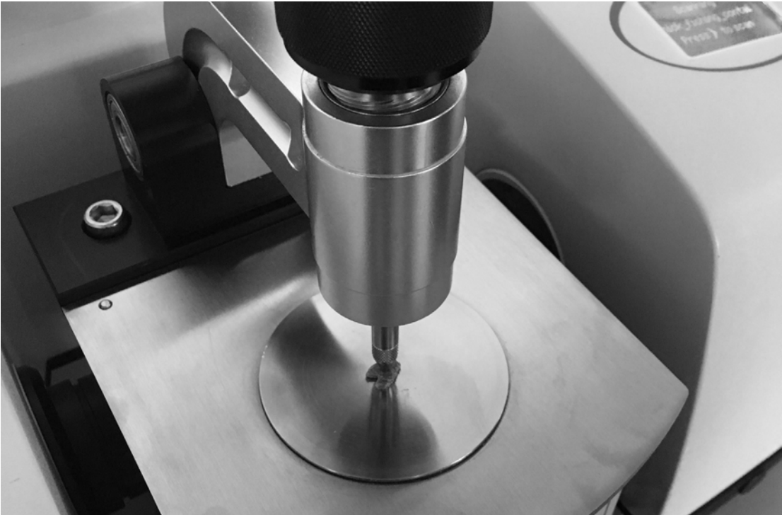
FTIR (Fourier-Transform Infrared Spectroscopy) instrument testing a plastic granule collected from Koster.
