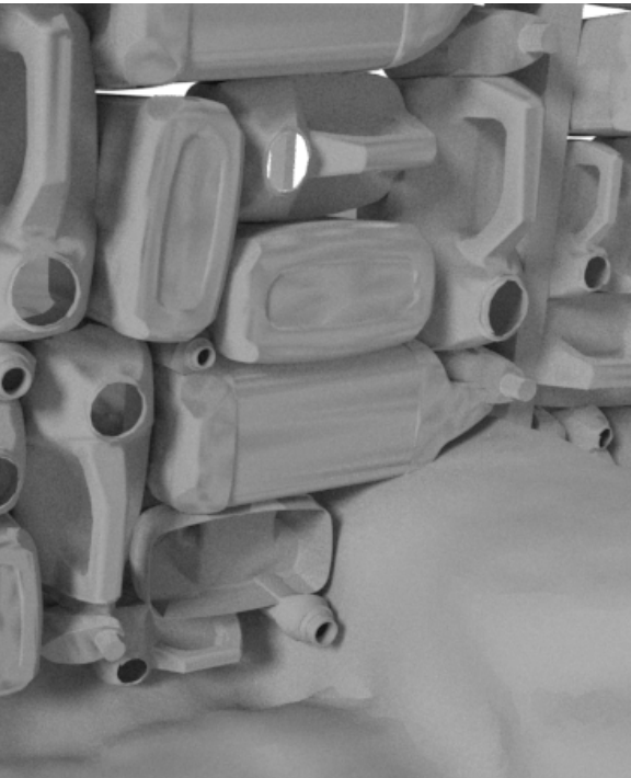
Testing different jerry can assembly systems. Stacking different sized jerry cans. Adapting them to the uneven ground where they will be positioned. Testing the lighting effect and different structural systems.
