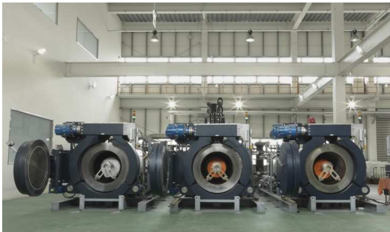
Figure 4: \text{SCCO}_2 dyeing machine produced by DyeCoo and installed in Yeh Group's facility in Tong Siang, Thailand. A machine is made up of three vessels and has a capacity of 2000 l, producing 1600 kg per batch.
