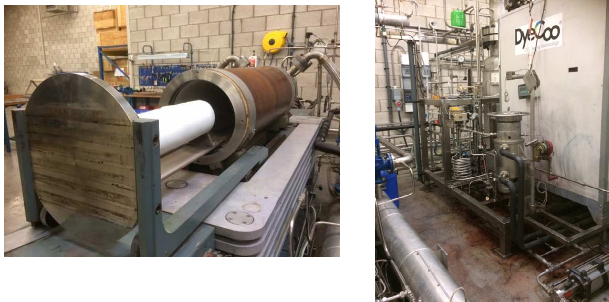
Figure 5: The 200-l dyeing vessel for R&D tests (left) and pressure and heating unit, recycle unit and control unit (right) in DyeCoo.
