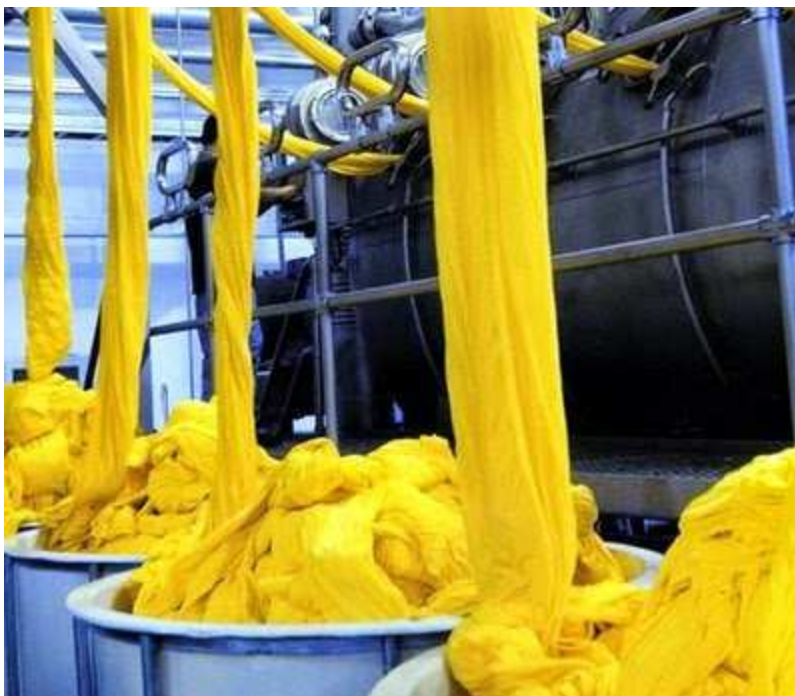
Figure 1: A water-based jet dyeing machine with external winch, dyeing fabrics in yellow. Source: http://textilelearner.blogspot.se/2011/12/dyeing-process-process-of-dyeing.html
