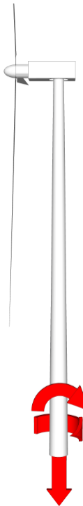
Figure 3.5: Tilting and torsional moments and normal force acting on the foundation. In this study the loads are provided by Vestas .
