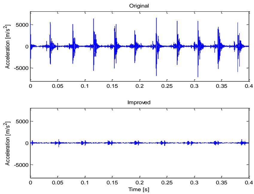
Figure 21 Vibration on original impact wrench and improved
