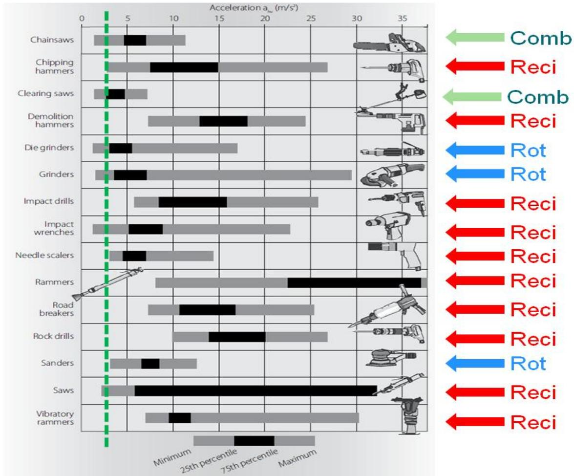
Figure 3 Machine types and their vibration level
