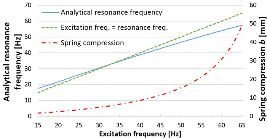
Figure 12 Analytical resonance frequency and spring compression versus excitation frequency
