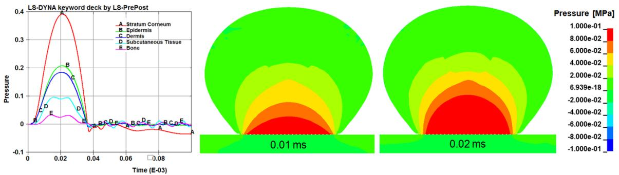
**Figure 9: Pressure distribution after load initiation and corresponding pressure propagation in the different finger sections for Variant A and B.**
