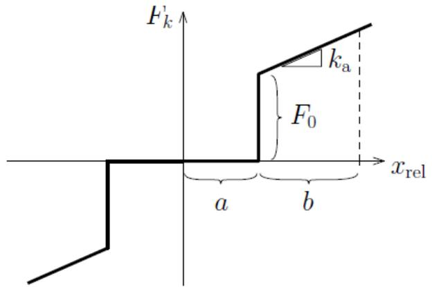
Figure 7 Nonlinear spring force in ATVA
