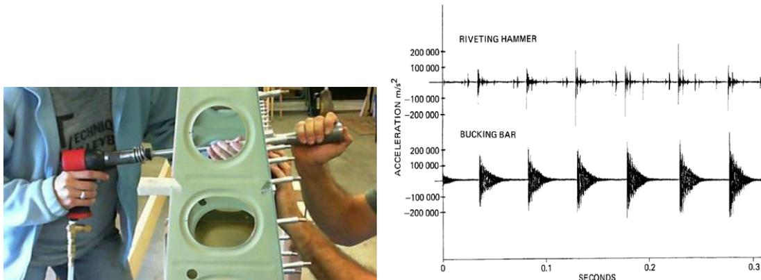
Figure 15 Riveting hammer (left) and bucking bar tool (right) and corresponding accelerations
