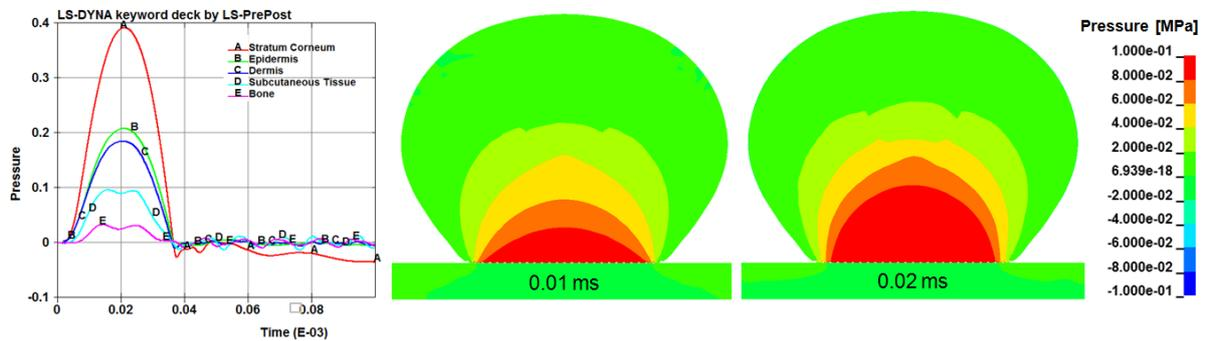
Figure 17: Pressure distribution after load initiation and corresponding pressure propagation in the different finger sections for Variant A and B.
