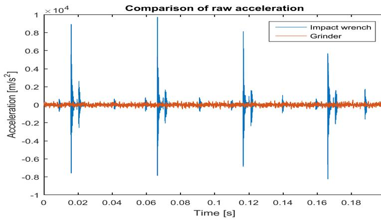
Figure 6 Grinder and impact wrench vibrations filtered at 30 kHz
