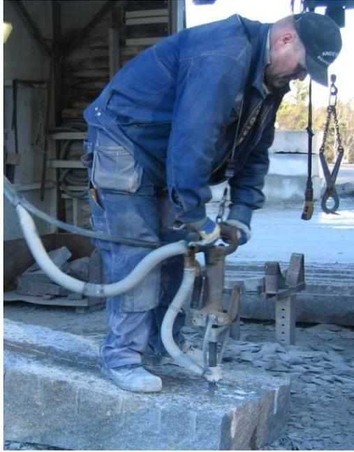
Figure 5 Chisel machine used in stone industry
