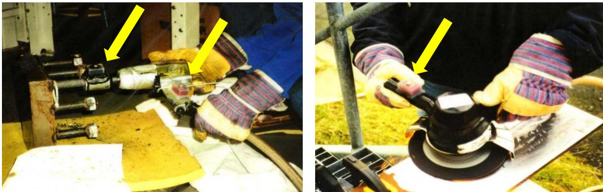
Figure 11 Blood container on impact wrench socket, handle and grinder handle
