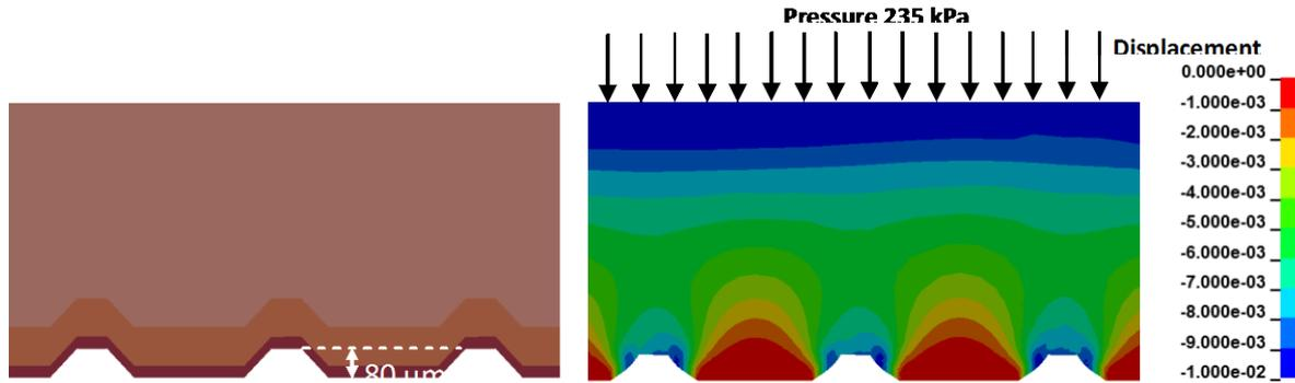
Figure 16 Unloaded geometry of the fingerprint (left) and numerical validation of the fingerprint distortion under constant pressure loading (right)
