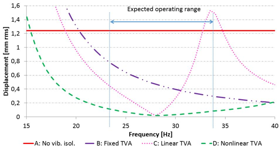
Figure 9 Vibration of the handle. Comparison between using the optimized Nonlinear TVA, the linear TVA tuned to 28 Hz, deactivated TVA (vibration isolation only) as well as no means of vibration reduction at all.
