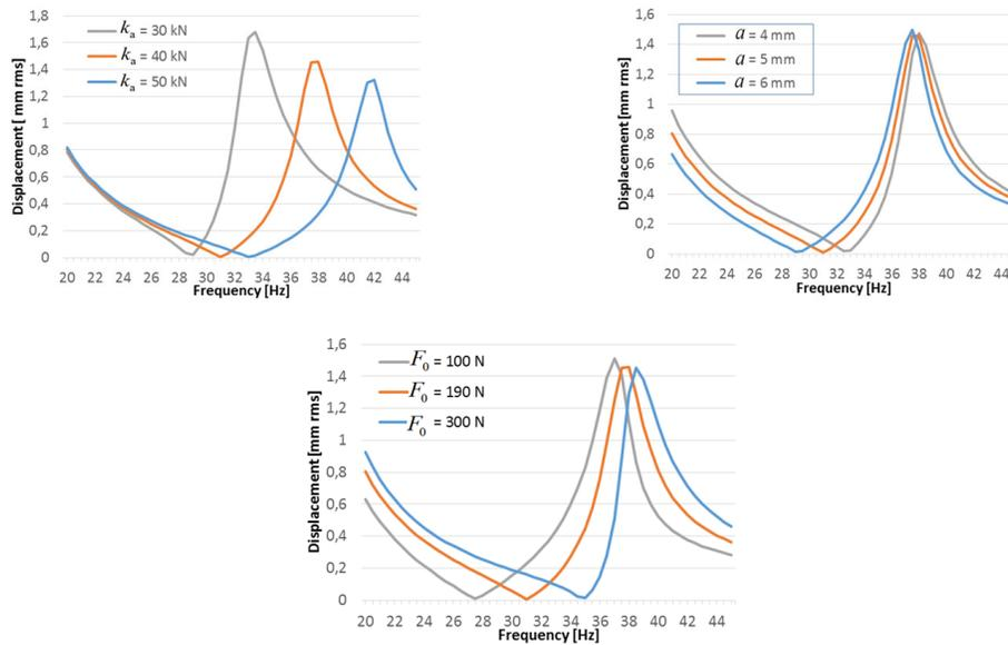
Figure 6: Vibration of the handle for different values of the NLTVA parameters. Only one parameter is varied at a time while other parameters are kept at their nominal values;  $k_a = 40$  kN/m,  $a = 5$  mm,  $F_0 = 190$  N.
