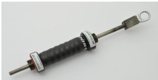
Figure 19 Vibration isolated anvil
