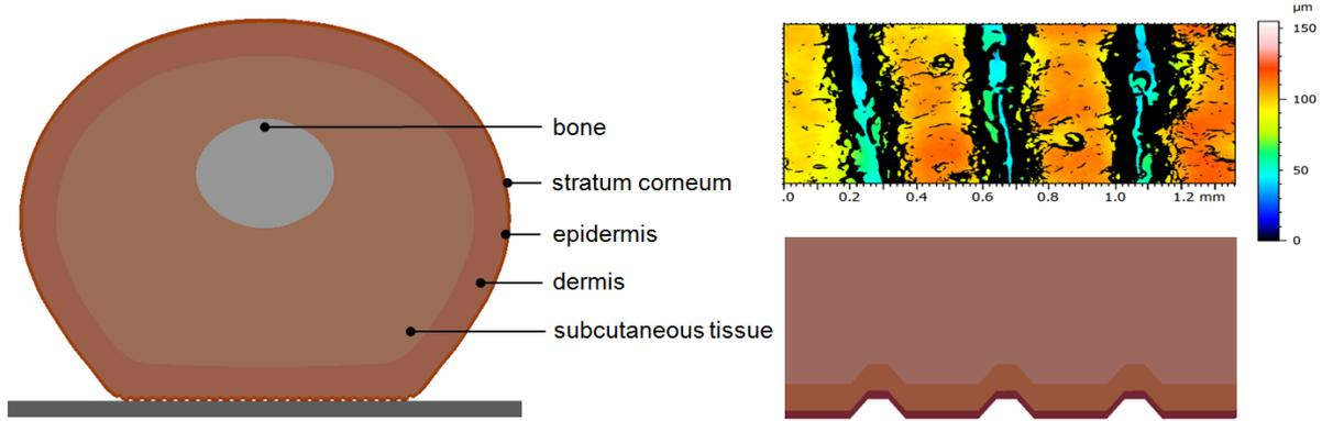
Figure 7: Numerical simulation model with experimentally validated geometry of the fingerprint
