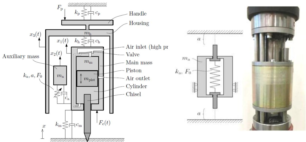
Figure 6 Left and middle, Engineering model of impact machine and auxiliary mass; Right, Prototype auxiliary mass
