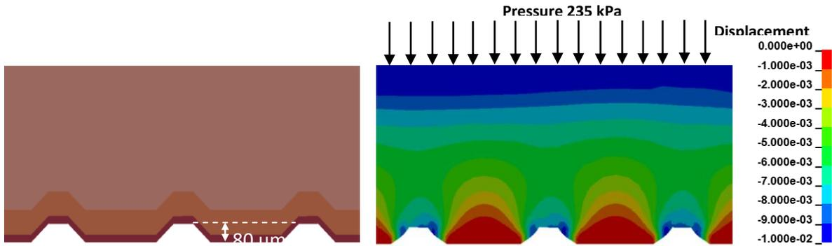
Figure 8: Unloaded geometry of the fingerprint (left) and numerical validation of the fingerprint distortion under constant pressure loading (right)
