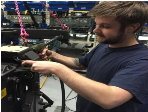
Figure 17 Tightening of screw joints with impact wrench and anvil
