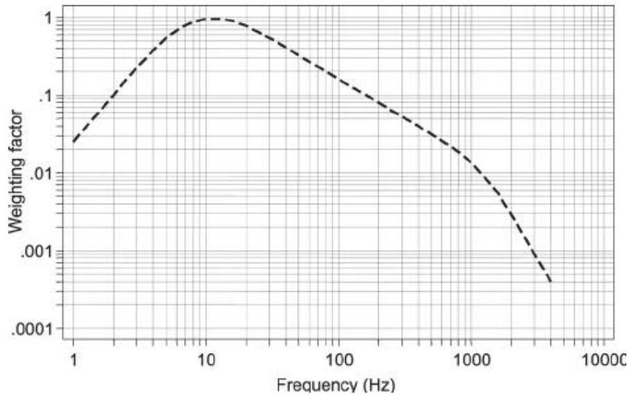
Figure 2 Frequency weighting curve for hand-transmitted vibration in ISO 5349-1:2001
