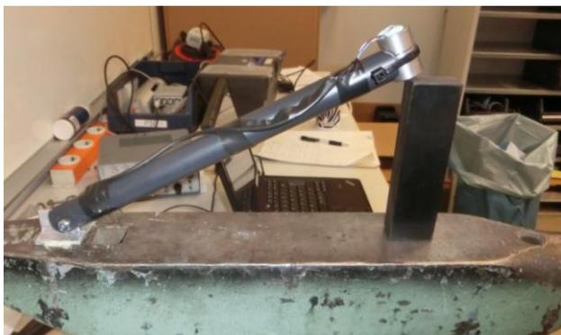
Figure 2 Test rig for accelerometer mounting evaluation
