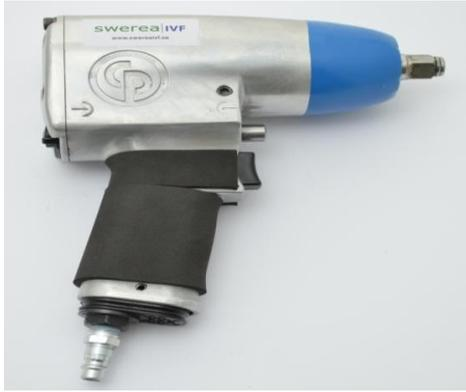
Figure 20 Vibration reduced impact wrench
