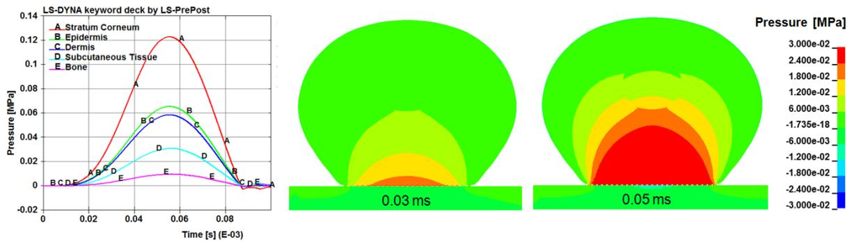
Variant B: Period of 0.01 ms and amplitude of 100 000 m/s<sup>2</sup>
