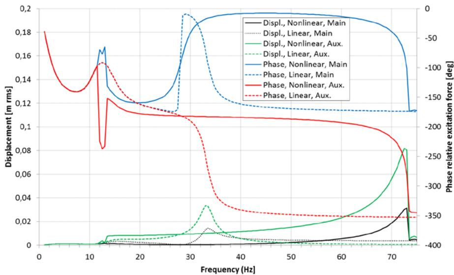
Figure 10 Phase and displacement for linear and nonlinear TVA
