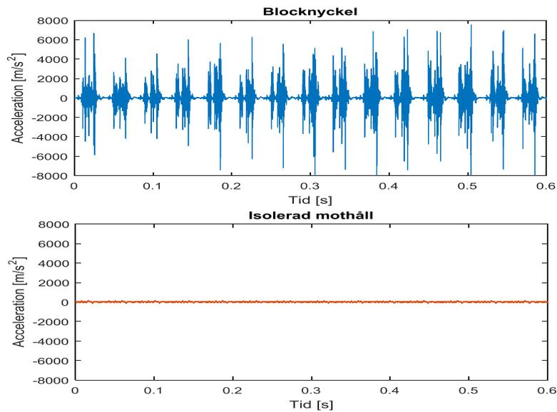
Figure 18 Vibration on original wrench anvil (top) and vibration isolated (below)
