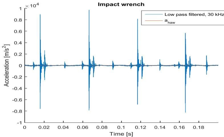
Figure 4 Impact wrench vibration before and after ISO 5349 filtering
