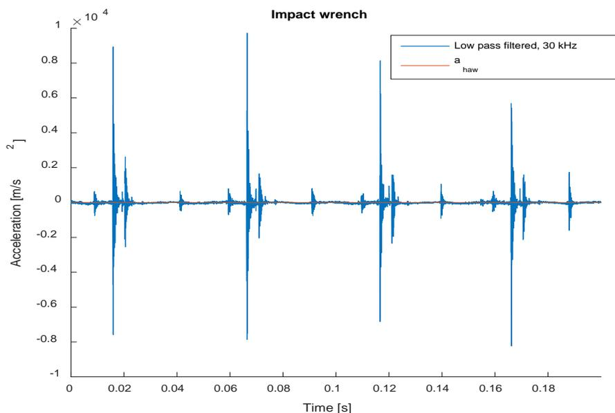
Figure 14 Vibration on impact wrench handle
