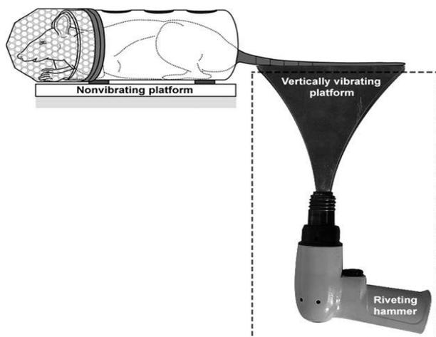
Figure 14 Test rig for rat tail
