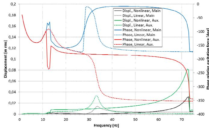
Figure 8: Phase and displacement for NLTVA and LTVA.
