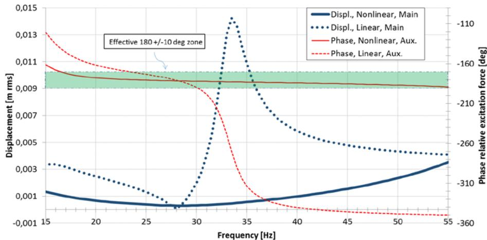
Figure 11 Phase and displacement for linear and nonlinear TVA, close up
