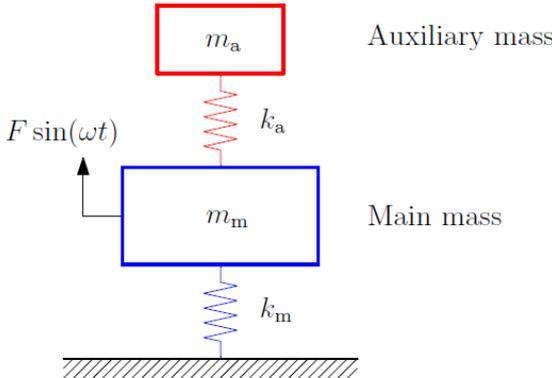
Figure 4, Tuned Vibration Absorber, [15]
