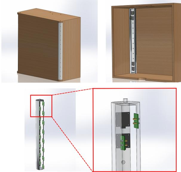
Figure 24: *Top, a section of the model from front and back views. The cylinder hosts the series of microblowers. Bottom, a zoom of the positioning of the microblowers.*
