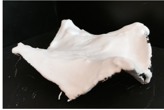
Figure 6-2. Double curved structure of nylon and plaster. (Photo: Ellen Simonsson)
