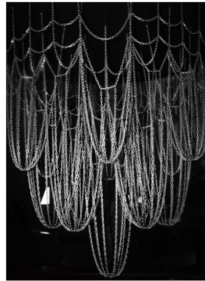
Figure 5-2. Above: Chains-net creating a natural form. This structure is a model for La Sagrada de Famila. (Photo: Ellen Simonsson).
