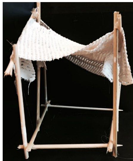
Figure 6-4. Twisted form of plaster bandage. (Photo: Ellen Simonsson).
