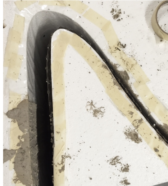
Figure 9-9. Deformation of formwork causing wider parts. (Photo: Ellen Simonsson)
