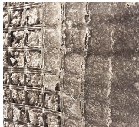
Figure 8-7. Detail showing how the concrete did not envelop the reinforcement. (Photo: Ellen Simonsson)
