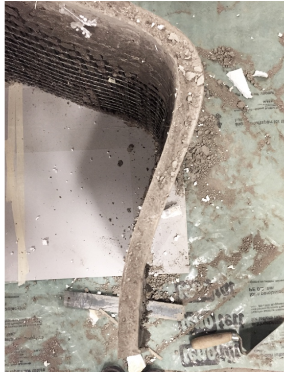
Figure 9-5. Not all reinforcement was enveloped by the concrete. (Photo: Ellen Simonsson)
