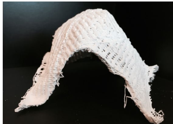
Figure 6-6. Shell of plaster bandages with four supports. (Photo: Ellen Simonsson)
