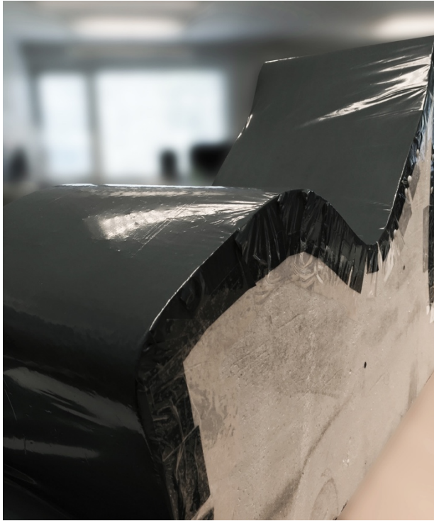
Figure 8-4. To left: Foam formwork with a layer of plastic. (Photo Ellen Simonsson).
