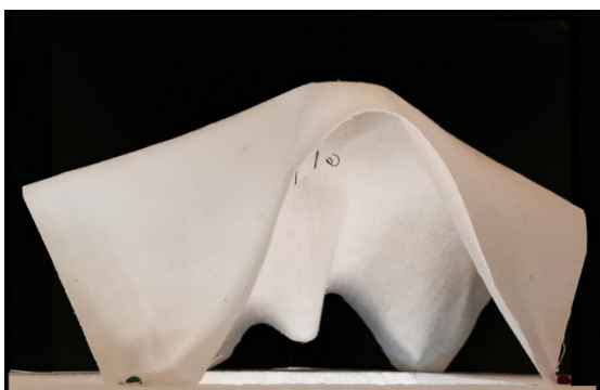
Figure 6-7. Same structure as shown in Figure 6-6 but upside down creates a shell in compression. (Photo: Ellen Simonsson).
