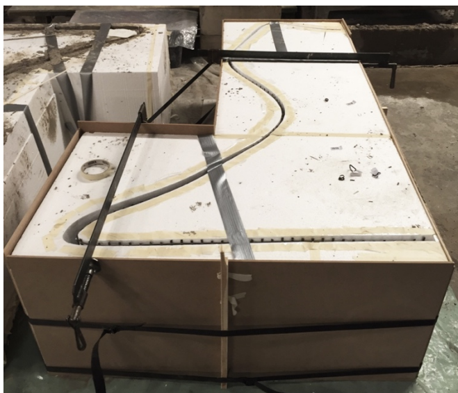
Figure 9-7. Formwork with 1 cm MDF to stabilize the form. (Photo: Ellen Simonsson)
