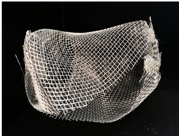
Figure 6-20. Double curved surface made of aluminum net. (Photo: Ellen Simonsson)
