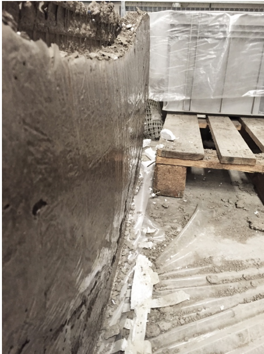
Figure 9-6. Some parts of the structure became twice as wide as expected. (Photo: Ellen Simonsson)
