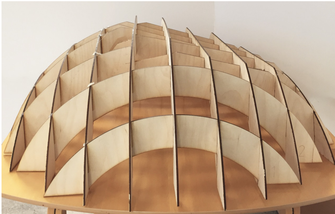
Figure 8-8. Wood form work. (Photo: Ellen Simonsson)
